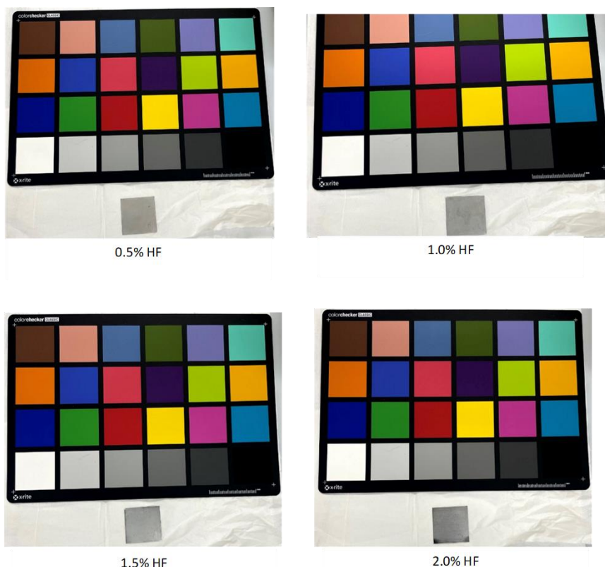
Figure 29. Comparison of the Set 5 post-etch samples and a color chart etched in 40wt% \text{HNO}_3 at varying HF concentrations. Etch time was 40 seconds.
