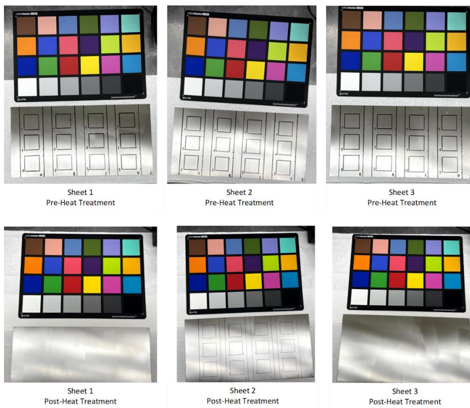
Figure 32. Sheets 1–3 before and after heat treatment between two Neolube-coated, stainless-steel sheets.
