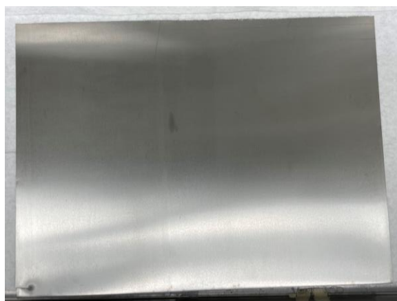
Figure 12. The Zr sheet following wet polishing at 3M.
