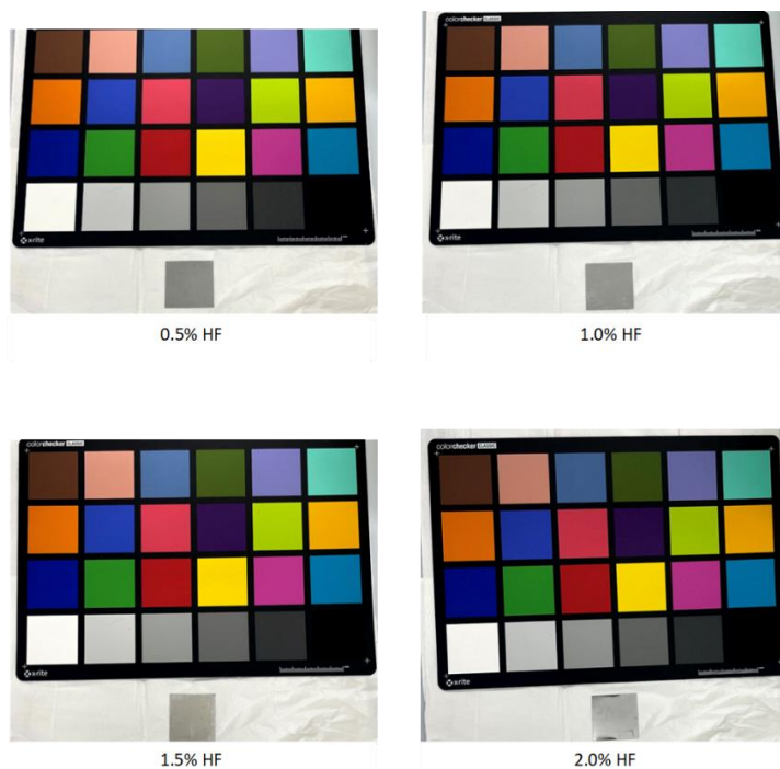
Figure 26. Comparison of the Set 4 post-etch samples and a color chart etched in 40wt% \text{HNO}_3 at varying HF concentrations. The etch time was 20 seconds.
