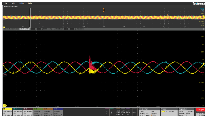
Fig. 13. Unsynchronized 3-phase inverter output waveform during hot-patch.
