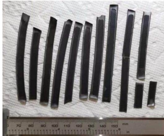
Figure 59. Photo of the PCES single cells of NiO-BCZYYb | BCZYYb | BCFZY0.1 made from RLRS prepared half cells and brushed cathode.
