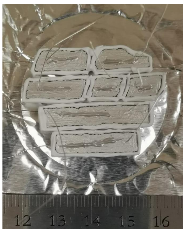
Figure 41. The photo of the combined single-cell prepared by one-step L3DP method. The total area is around 6.6 cm 2 .
