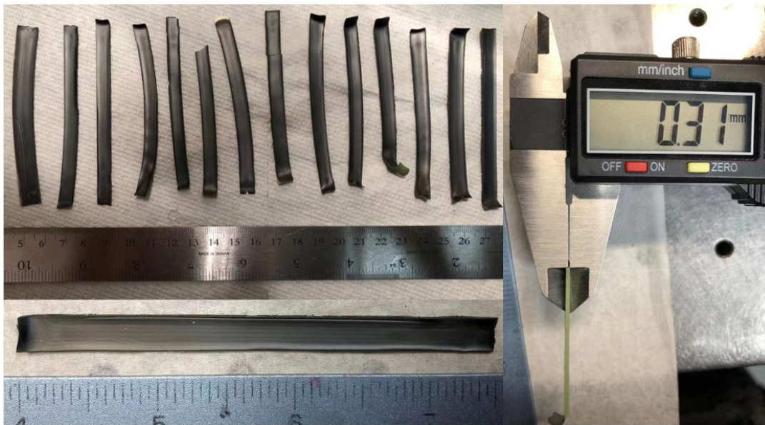
Figure 58. Photos of half-cells prepared by RLRS using 250W CO 2 laser
