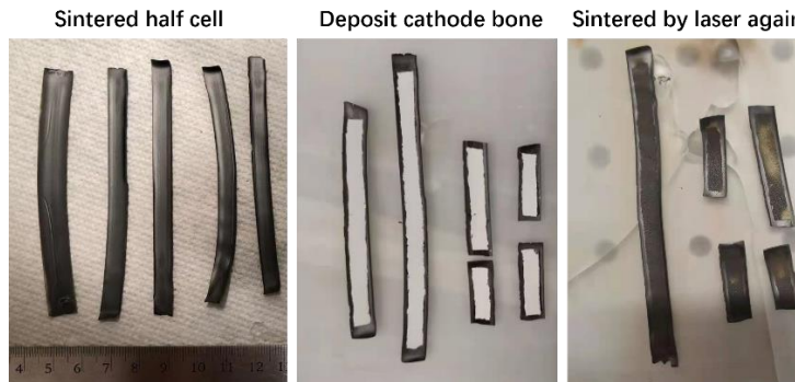
Figure 64. The photos of the half cells, single cells with green cathode scaffold, and sintered single cells Cell 3: 40wt% BCZYYb + 60wt% NiO | BCZYYb +1wt% NiO | BCZY63+BCFZY0.1 (0.32 cm 2 ) by complete laser processing
