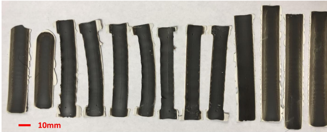
Figure 23. Summary optical photo of half cells fabricated by L3DP.
