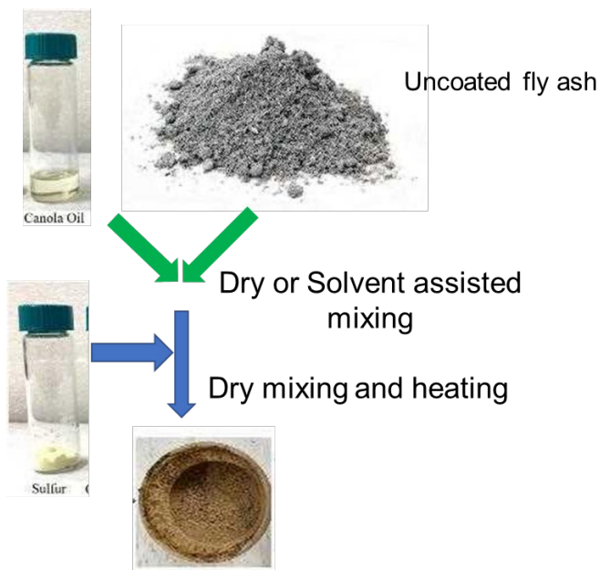
Figure 10. SuMo fly ash generation by sulfurization of vegetable oil (SVO) coated fly ash
