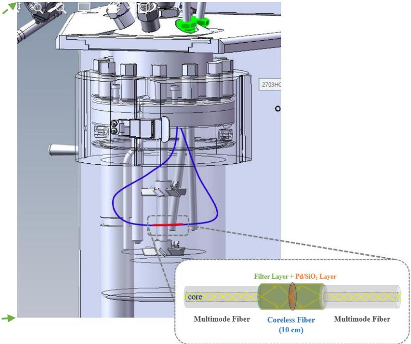
H<sub>2</sub> sensor installed inside
