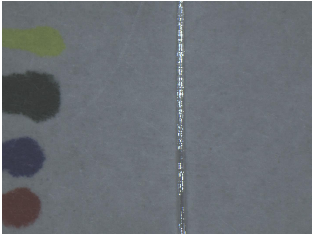
Figure 6. Microscope image of ~330 \mu\text{m} diameter Ce:YAG fiber. The length shown in this image is roughly 1.2 cm.
