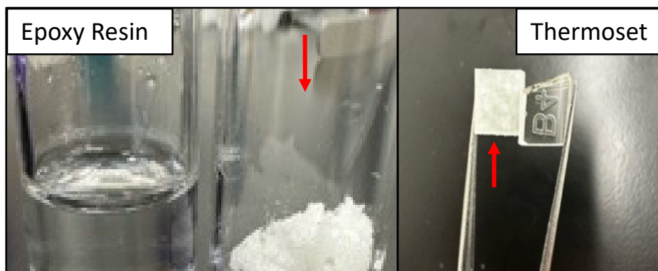
Figure 2. Picture of liquid and crystalized epoxy resin and cured thermoset with and without integrated epoxy crystals. Crystalized epoxy resin and crystal integrated thermosets are marked with red arrows.
