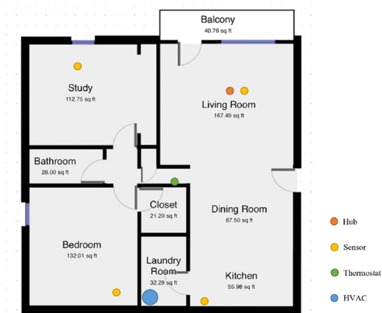
Figure 12. Floorplan and system installation
