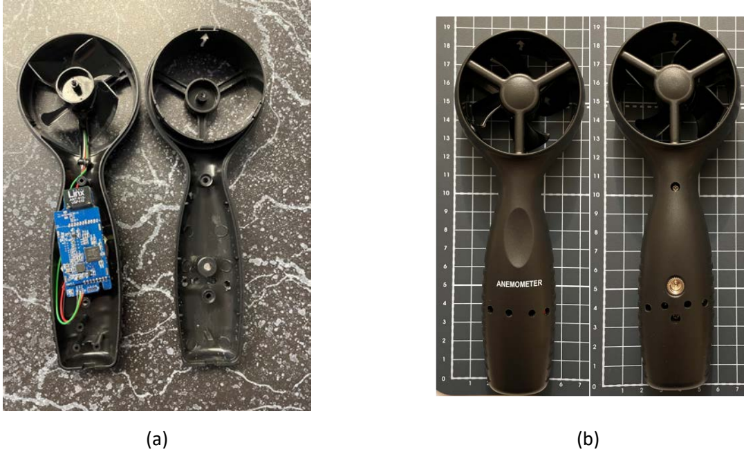
Figure 17. THSP unit housed within the airflow sensor handle
