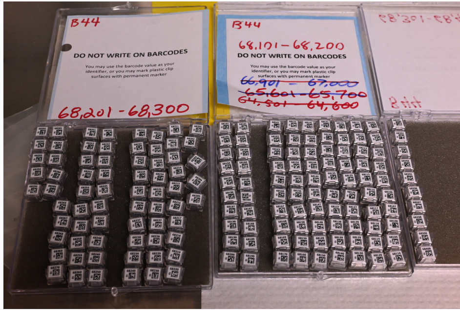
Figure 3.5: An assortment of \text{CaF}_2 TLDs used for the photon dose measurements at different distances.
