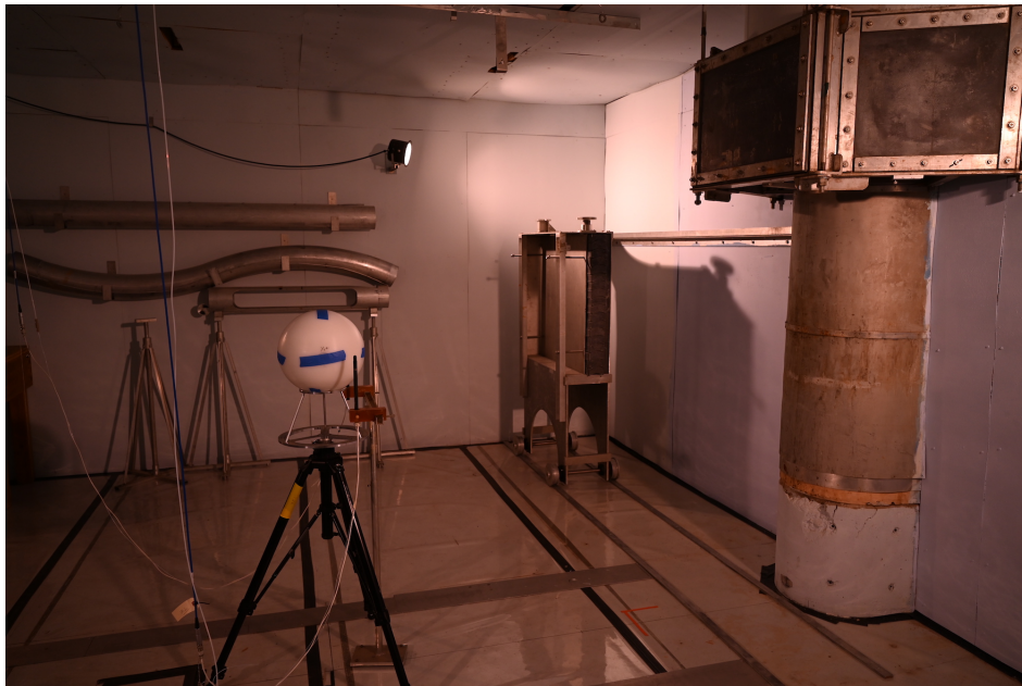
Figure 3.1: PNS sphere sitting on an aluminum stand and mounted on top of a tri-pod in ER1. The walls were painted with a gadolinium paint and the semi-circle portion of the wall was a cadmium lining on top of the painted wall.
