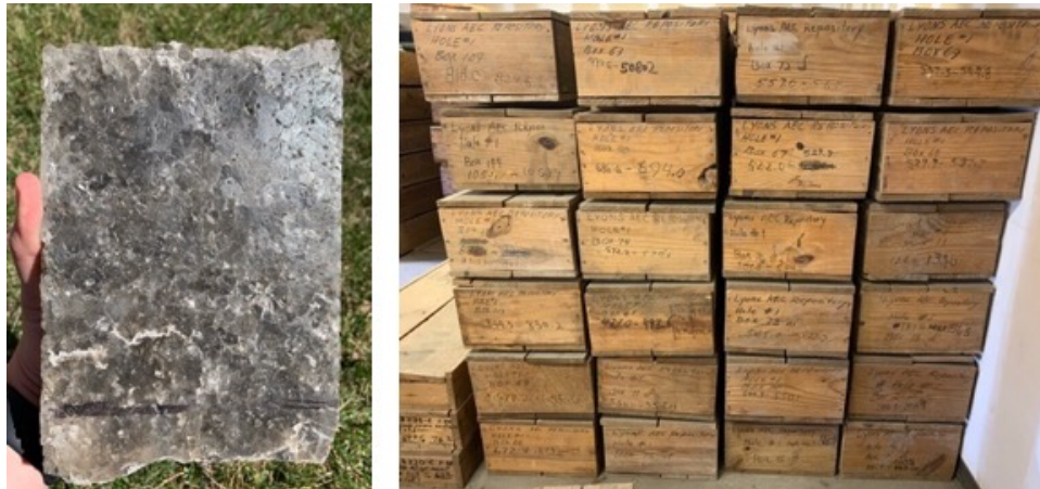
Figure 19: Hand-sample and core boxes of Kansas salt collected as part of scoping studies for a possible nuclear waste repository near Lyons, Kansas, in the 1960s by the US Atomic Energy Commission.
