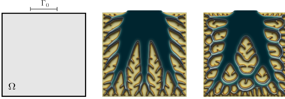
FIGURE 6.5. Left: Depiction of the subsets of the domain boundary \partial\Omega for the boundary conditions for the heat field u in (6.5). We define u = 0 on \Gamma_0 and \nabla u \cdot \mathbf{n} = 0 on \partial\Omega \setminus \Gamma_0 . Middle: Reference density field \bar{\rho} for the solution of the deterministic thermal compliance optimization problem (6.6) with f \equiv 1 everywhere in \Omega . Right: The filtered density \tilde{\rho} for the solution of the expected value thermal compliance optimization problem (6.6) with f given by (6.5). The presence of closed-loop branches in the optimal solution on the right indicates a preference for balancing the heat locally and transferring only the excess unbalanced heat to the external environment through \Gamma_0 .
