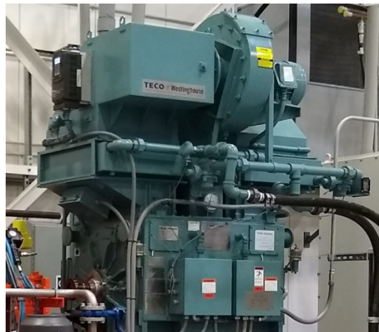
Figure 5: The prototype high speed induction machine with a flanged shaft prepared for factory acceptance tests.
