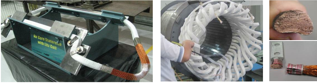
Figure 6: Litz wire coil sample, stator with Litz wire and Litz wire joint tests
