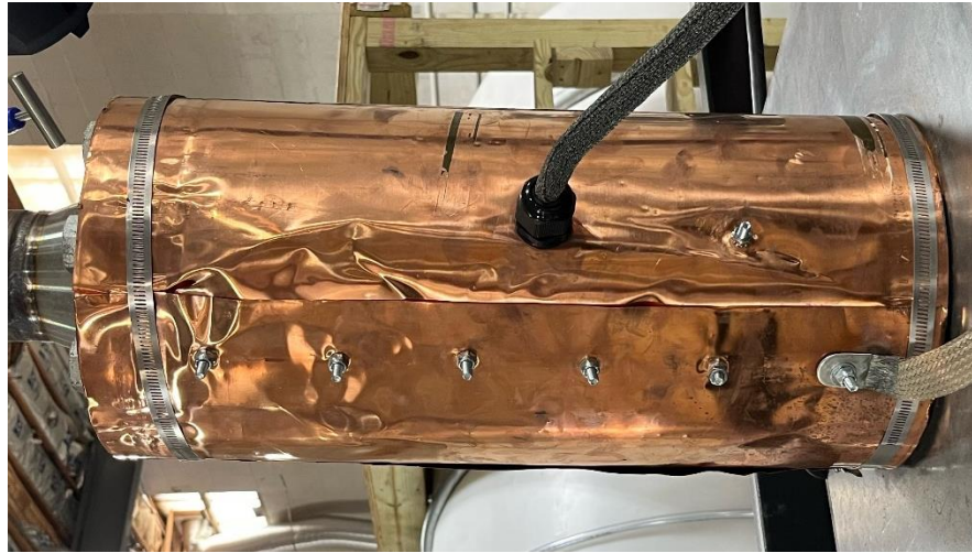
Figure 8: Sensor cable shielding and ground braid
