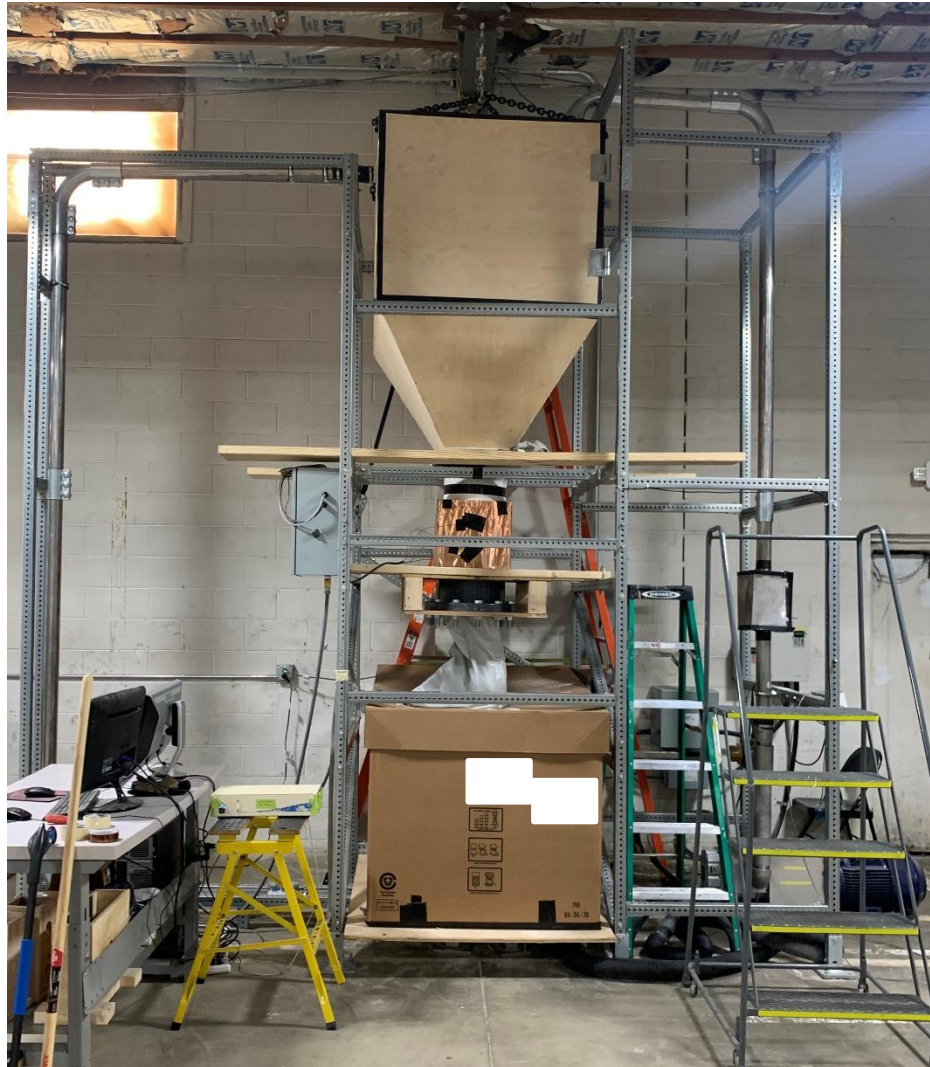
Figure 25: Gas-solid flow loop for studying ECVT mass flow measurement of solids content.
