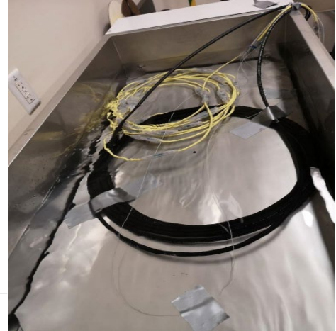
Figure 2.18 The water bath test setup for the temperature change test. 1 m, 2 m and 10 m sections of optical fiber was merged in the water to be heated with accurate temperature control. The length between 1 m and 2 m is about 5m and the length between 2 m to 10 m is about 40m.
