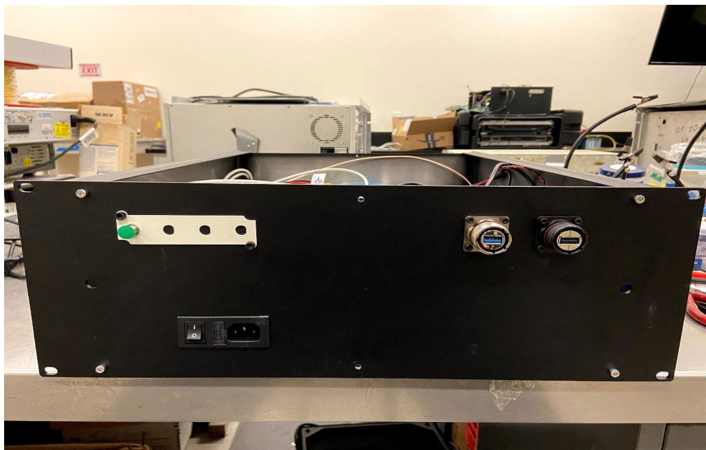
Figure 2.14 The front panel of the enclosure. This front panel includes FC/APC connector, power switch and USB connectors.
