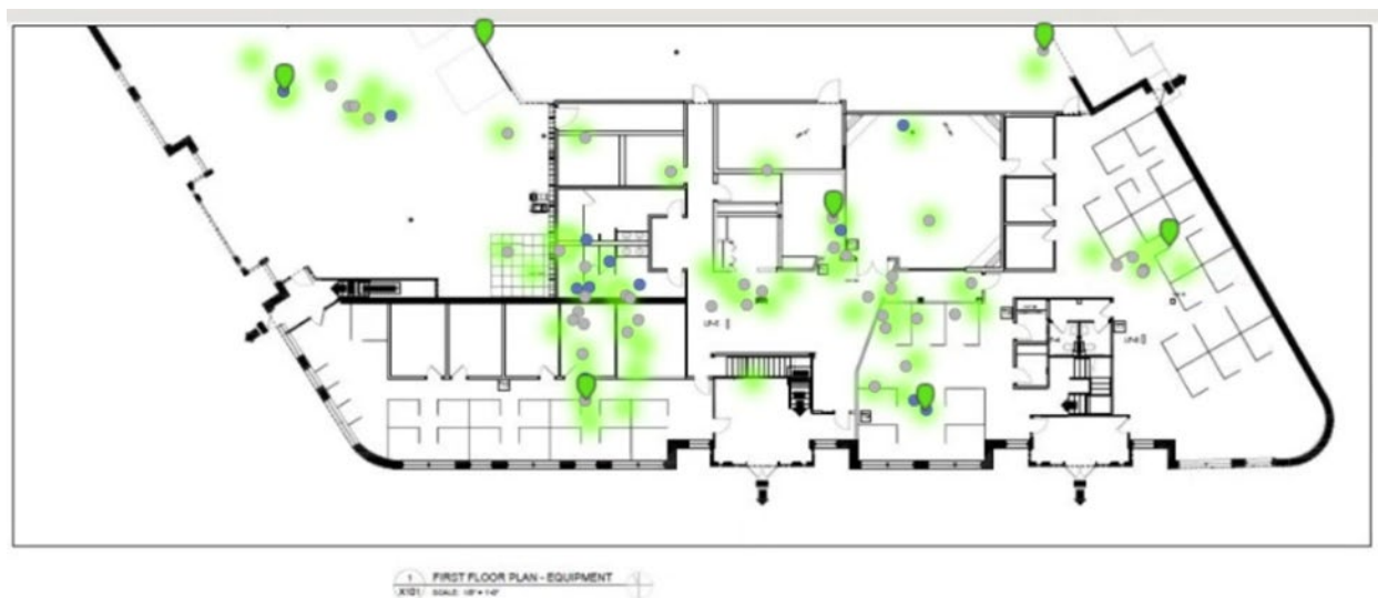
Figure 11. PTI floorplan from the Meraki dashboard showing locations of detected Wi-Fi enabled devices
