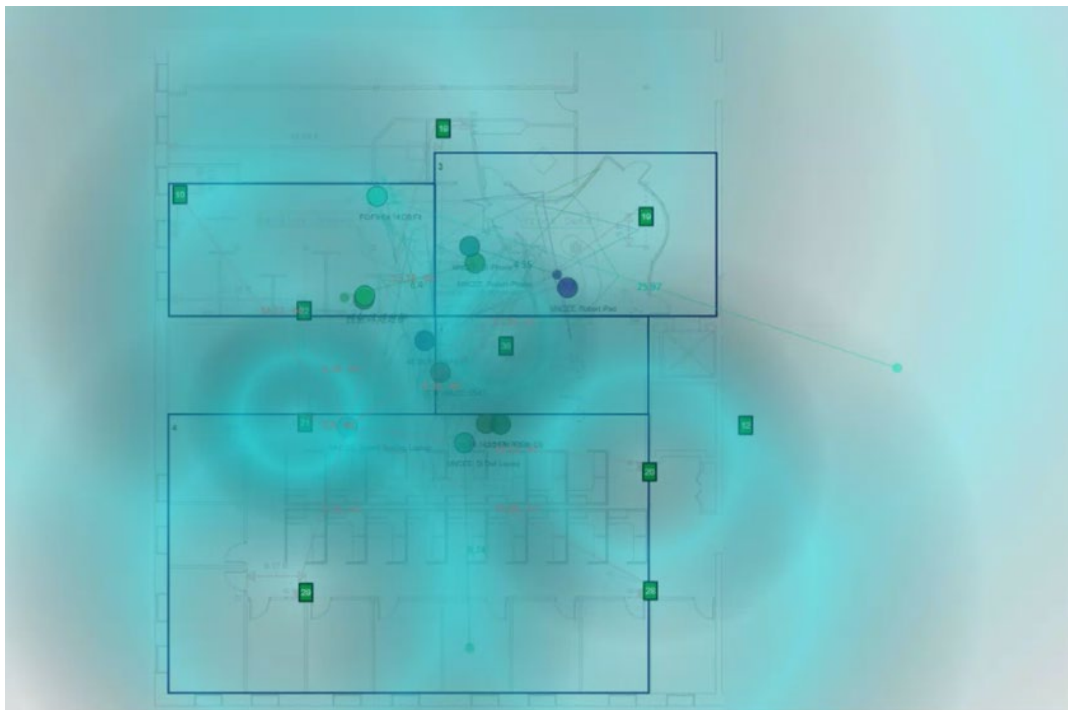
Figure 8. Heat map of the predicted location of a signal in the CEE Lending Center and reception area
