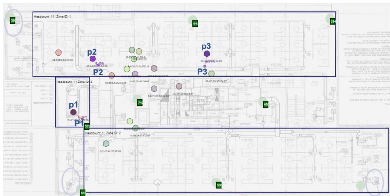
Figure 26. Comparison of LDA-calculated reference point locations with actual locations at the Slipstream offices
