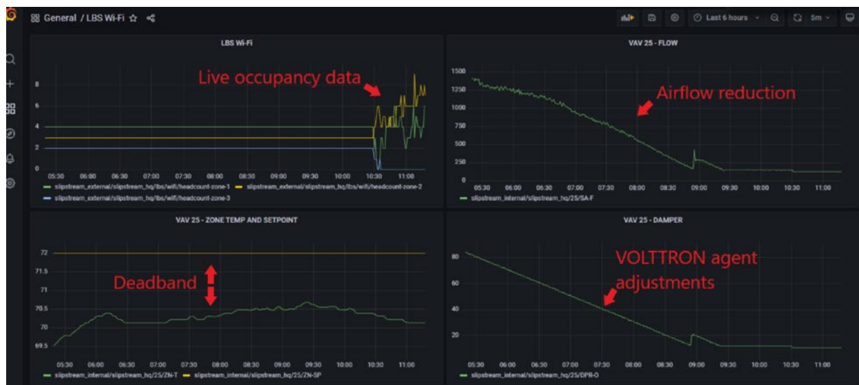
Figure 36. VOLTRON agent at work adjusting the HVAC system VAV box zone
