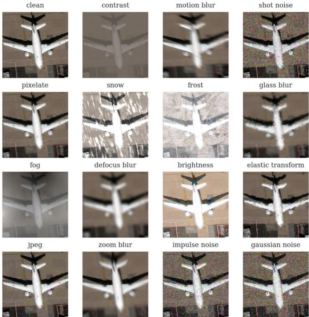
Figure 9: RGB corruptions of a RarePlane chip from our test set.
