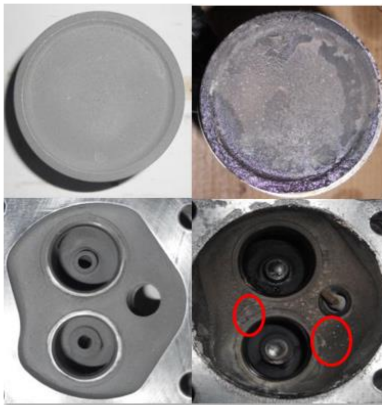
Figure 16.8. Piston and Head coated with the RC Coating Before (Left) and After (Right) 400 hours of genset durability testing. Although the coating remained in good condition on the piston, a large amount of carbon deposits formed on its surface. The head remained in fair condition as there were two areas where minor flaking occurred.
