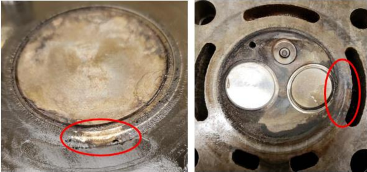
Figure 15.2. Head Gasket Leakage.
