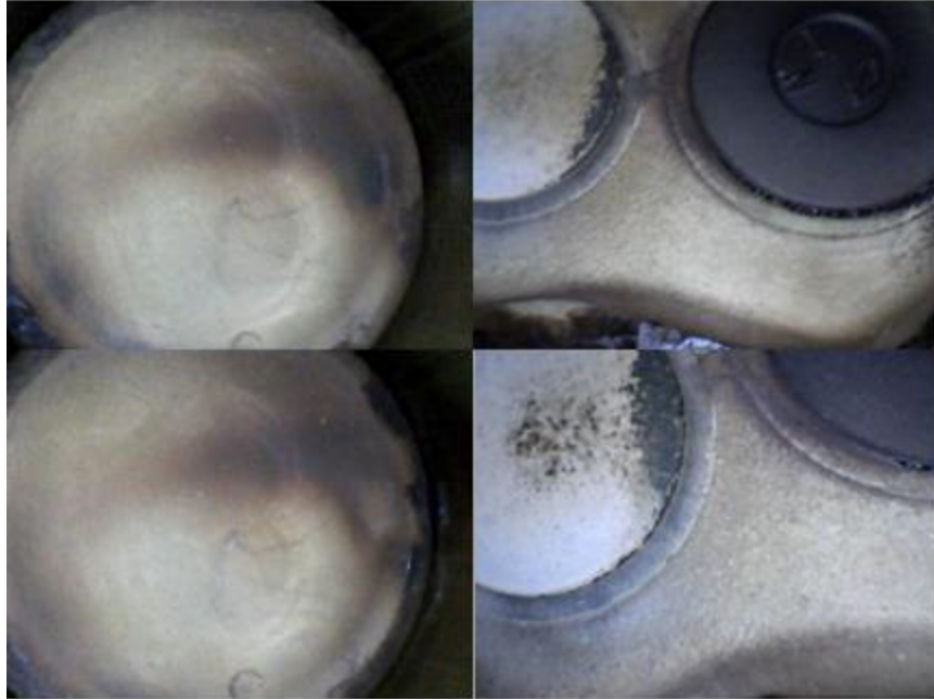
Figure 28.10. Set 2 borescope pictures after 28 hours (top) and after 83 hours (bottom). Coating remains in good condition with no signs of delamination.
