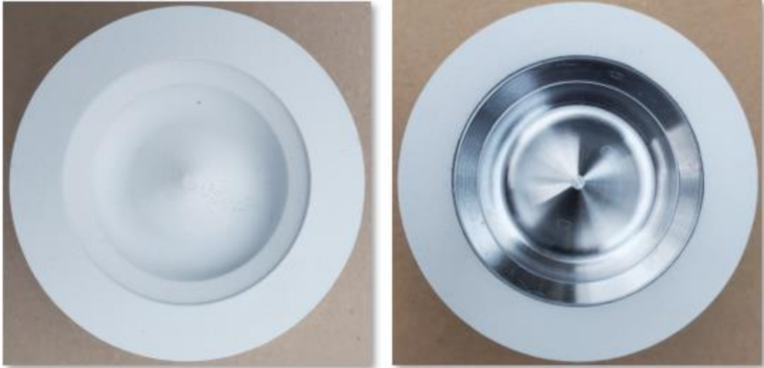
Figure 29.2. Piston coated with PSZ on entire profile (Left) and piston coated with PSZ on squish area only (Right).
