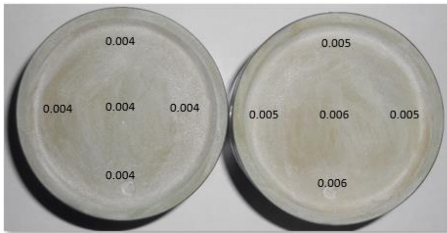
Figure 28.7. Piston 1 (Left) and Piston 2 (Right) coated with the SPC Coating + Sealer before 100-hour durability testing (measurements in inches).
