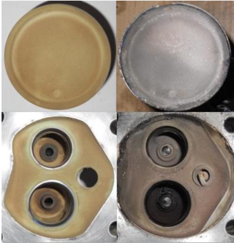
Figure 16.9. Piston and Head coated with the PC Coating Before (Left) and After (Right) 400 hours of genset durability testing. The coating on both remained in good condition throughout testing without any notable deterioration.
