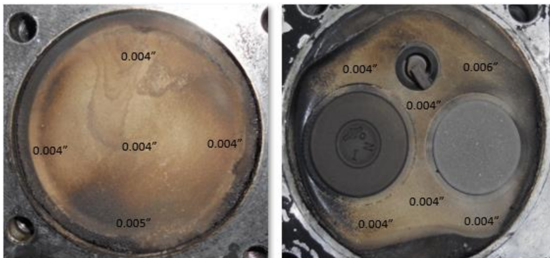
Figure 28.11. Set 1 (SPC Coating + Sealer) after 100 hours of durability testing (measurements in inches).
