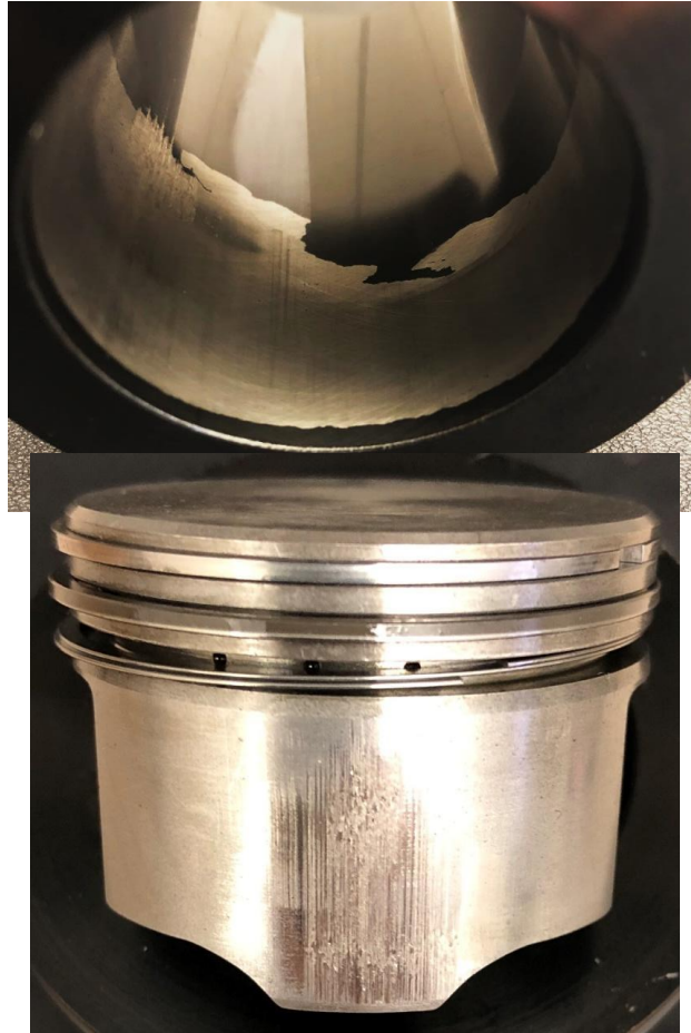
Figure 18.1. DLC Coated Sleeve Failure and Piston Damage.
