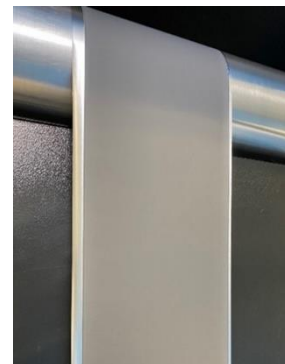
Figure 5. Slurry cast NMC cathode by R2R process
