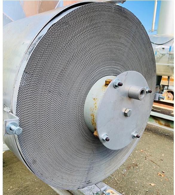
Figure 41. Example of wound crimped ribbon style flame arrestor that can be used in various natural gas system components including flares, from [128].
