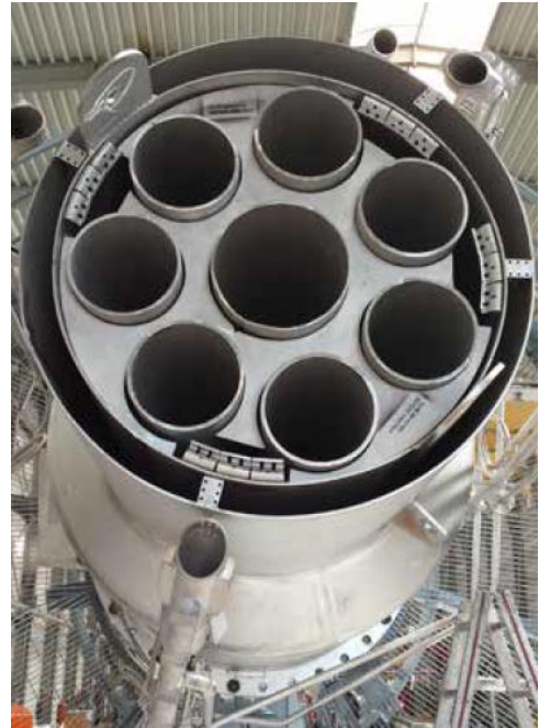
Figure 36. Air-assisted flare tip similar to steam assisted designs, from [107].
