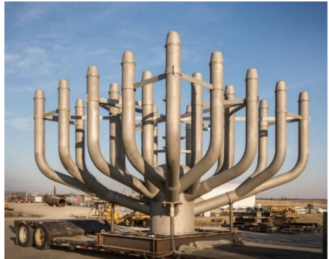
Figure 24. Multipoint sonic flare tip, from [105].
