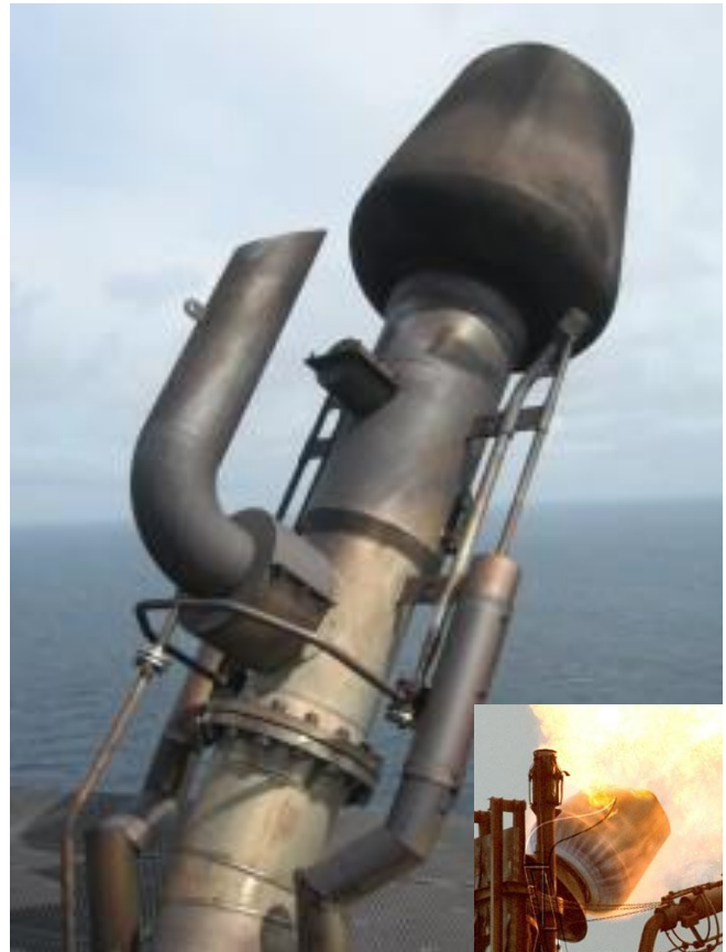
Figure 26. Coanda flare tip, from [100].
