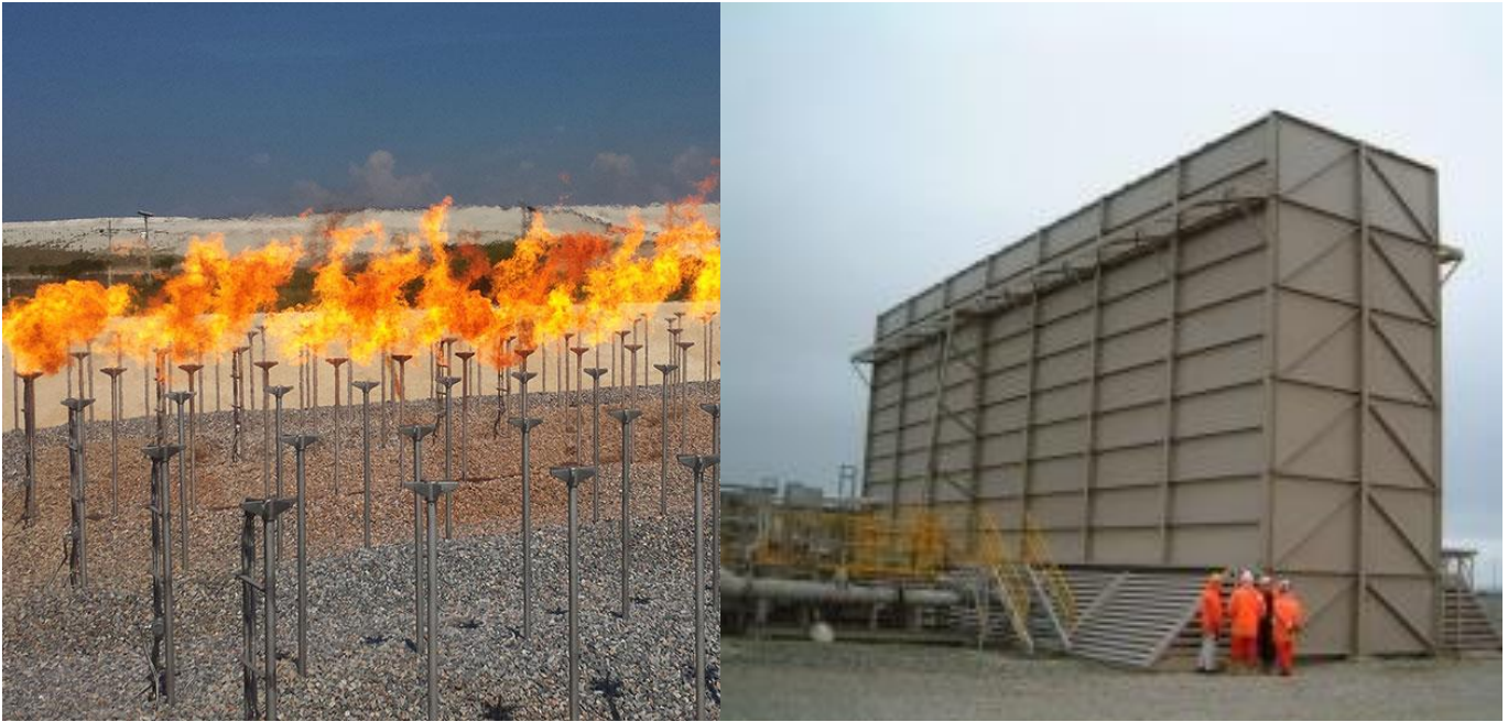
Figure 19. Open ground flare (left) [79] and enclosed ground flare (right) [77].
