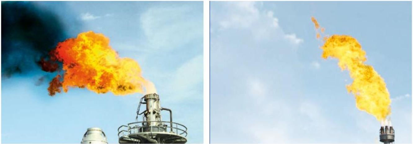
Figure 29. Impact of steam injection on smoke formation, without (left), with (right), from [76].
