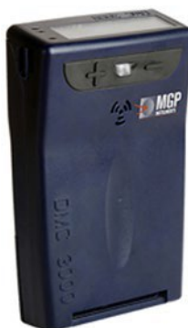
Figure 21: Mirion Technologies DMC-3000 Dosimeter Used at Y-12
