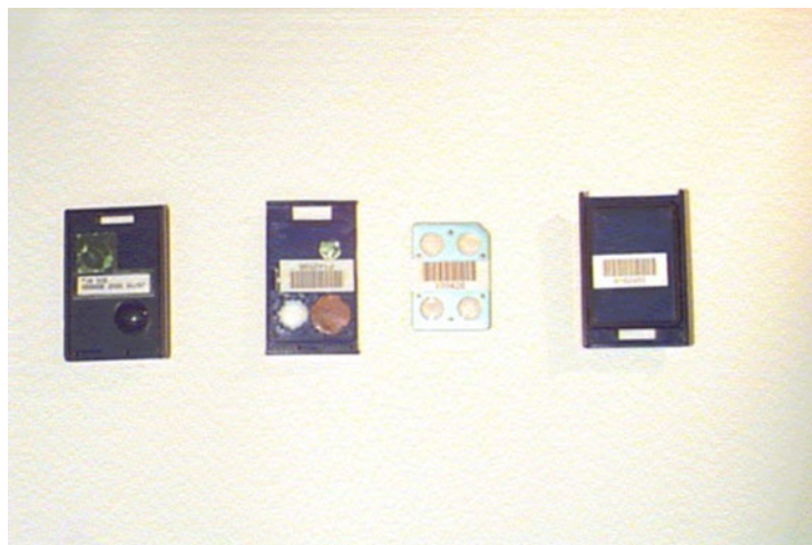
Figure 19: Harshaw 8805 Beta-Photon Dosimeter Used at Y-12
