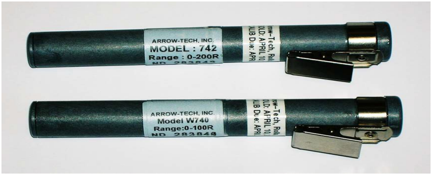
Figure 17: Examples of Arrow-Tec Direct Reading Pencil Chambers
