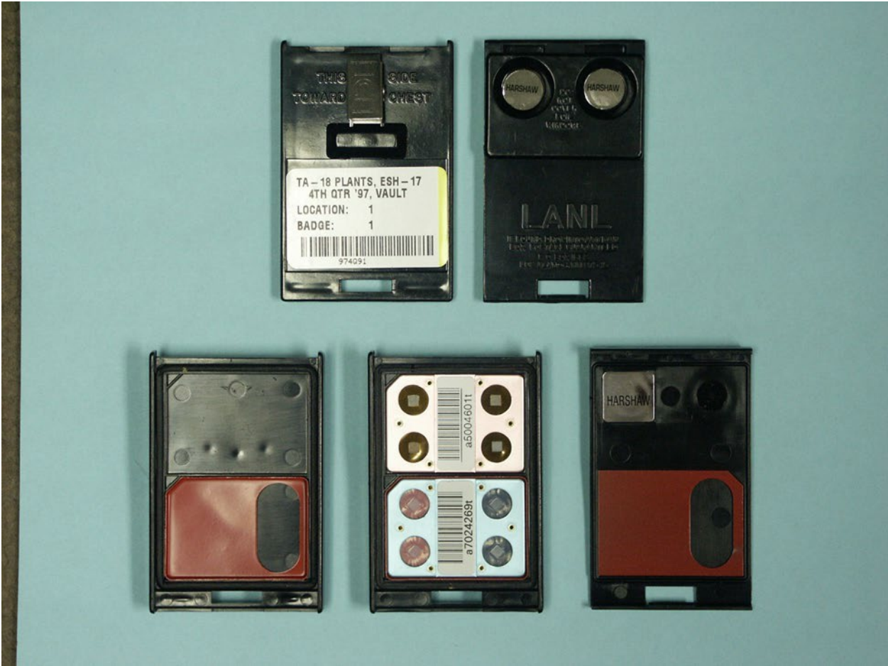
Figure 13: LANL 8823 Whole-Body Dosimeter
