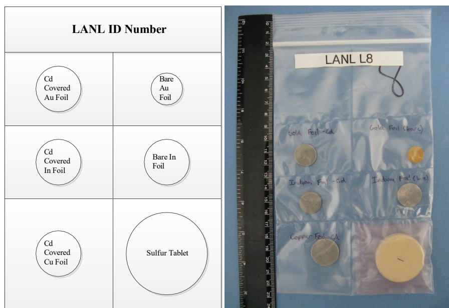
Figure 14: Los Alamos Criticality Intercomparison Dosimeter
