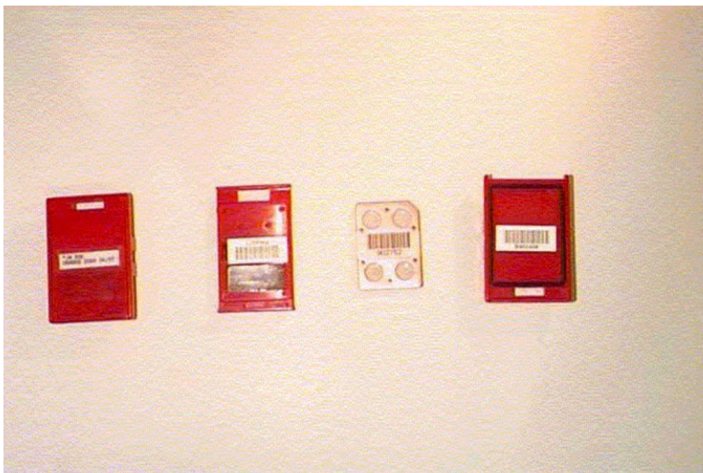
Figure 20: Harshaw 8806 Neutron Dosimeter Used at Y-12
