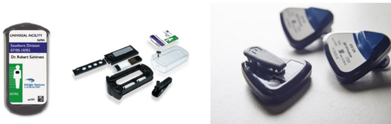
Figure 23: Landauer InLight and Mirion Instadose+ photon dosimeter
