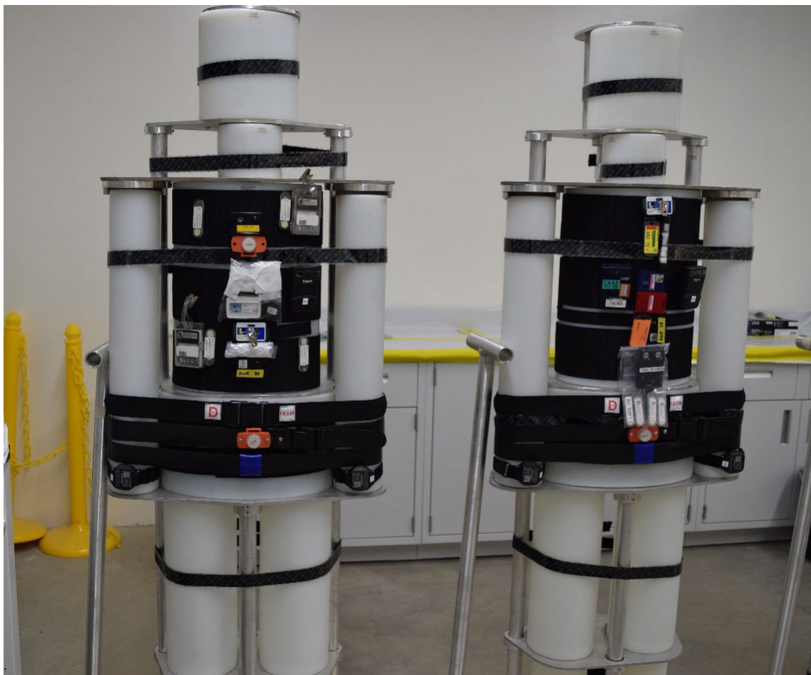
Figure 3: BOMAB on stand with dosimetry placed on front and backside.
