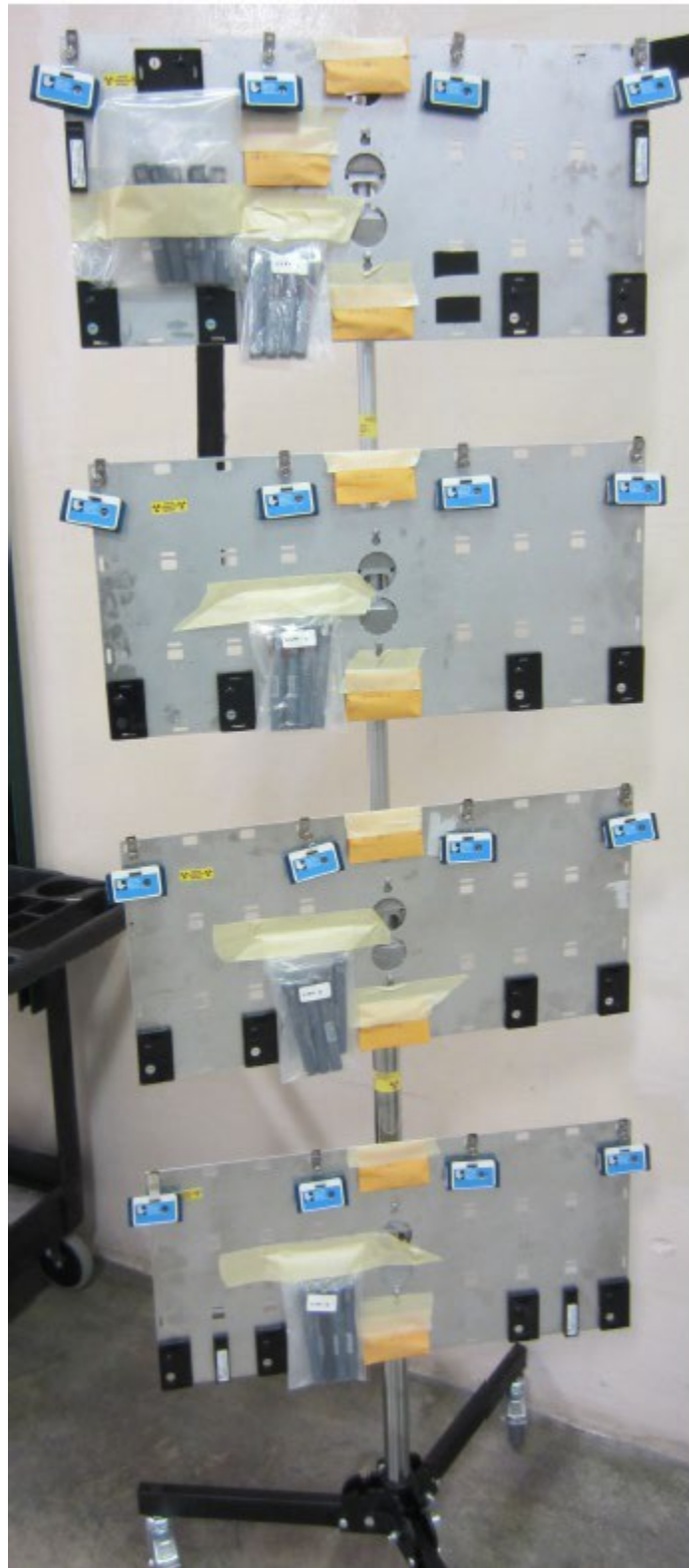
Figure 4: Dosimetry placed on aluminum plates on a rolling stand.
