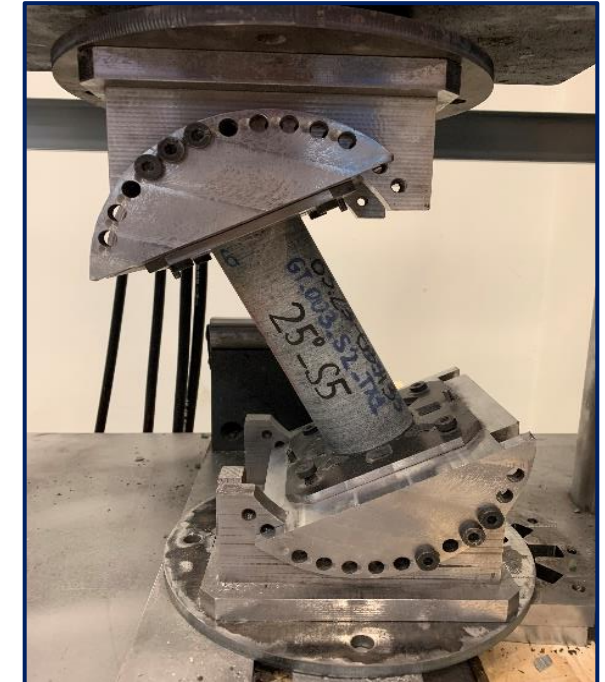
Rock sample testing at 25^\circ inclination using C-CAST system.
