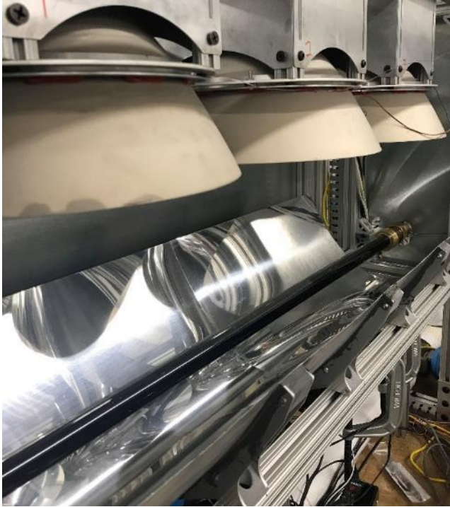
Figure 55: Sub-Scale LTS with the Solar Simulator Filled with Acid Black 52 Dye Figure 56: Boiling of the Dye Working Fluid During Application of Simulated Solar Energy
