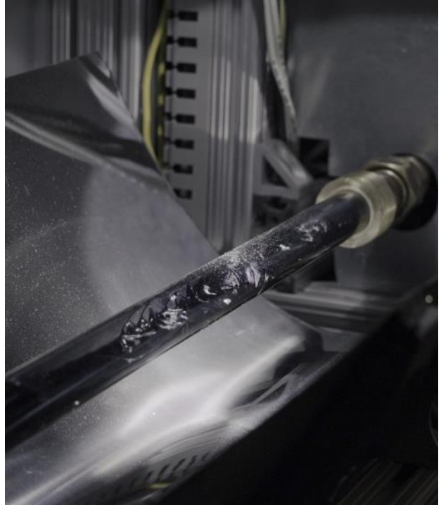
Figure 55: Sub-Scale LTS with the Solar Simulator Filled with Acid Black 52 Dye Figure 56: Boiling of the Dye Working Fluid During Application of Simulated Solar Energy
