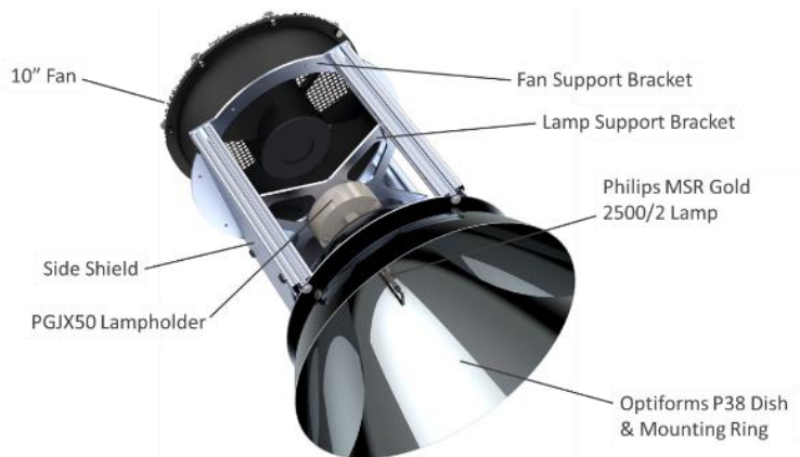
Figure 49: Metal Halide Solar Simulator Lamp Assembly Design
