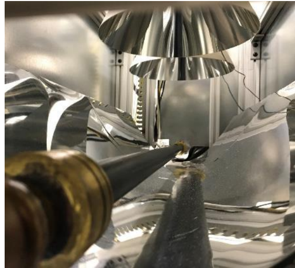
Figure 57: Sub-Scale LTS with Solar Simulator and Copper Receiver with High-Absorptivity Surface Coating.
