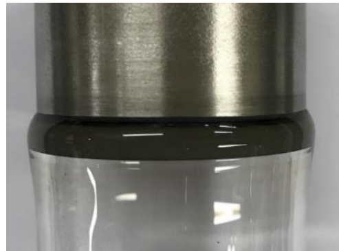
Figure 20: Borosilicate Glass-Kovar Joint Fabricated Using the Graded Seal Method.
