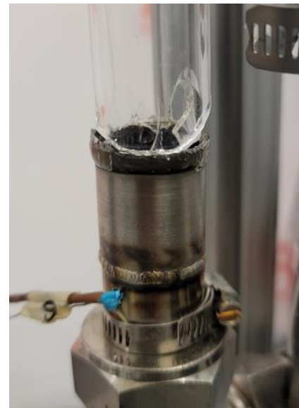
Figure 33: Broken Kovar-Glass Joint After \sim 5,000 Thermal/Pressure Cycles
