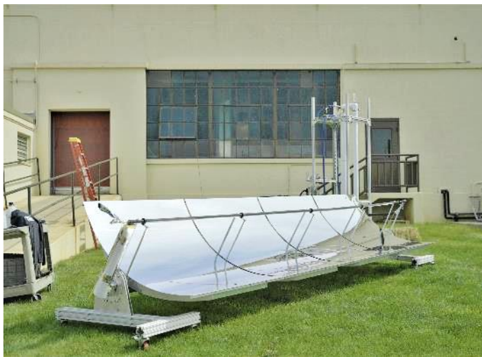
Figure 77: Full-Scale Parabolic Trough Solar Collector LTS During Testing
