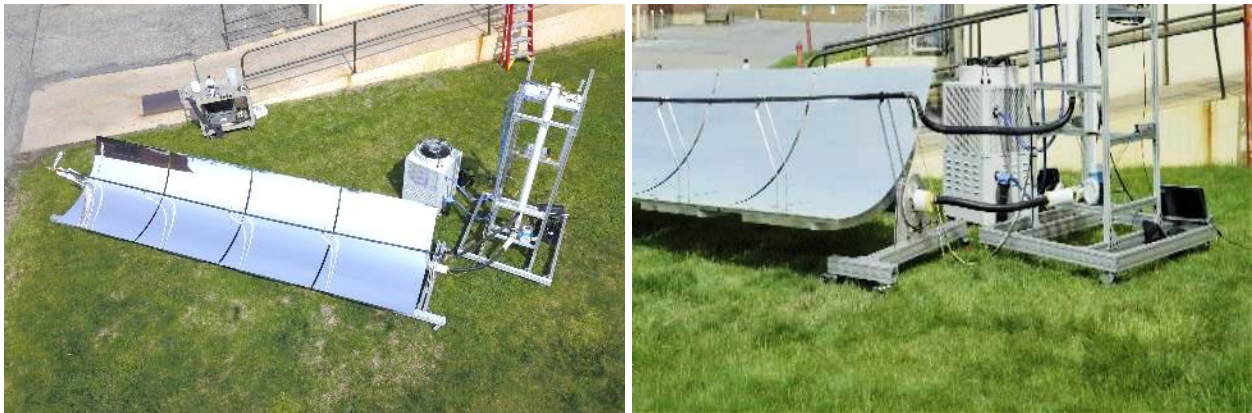
Figure 76: Full-Scale Parabolic Trough Solar Collector LTS During Testing
