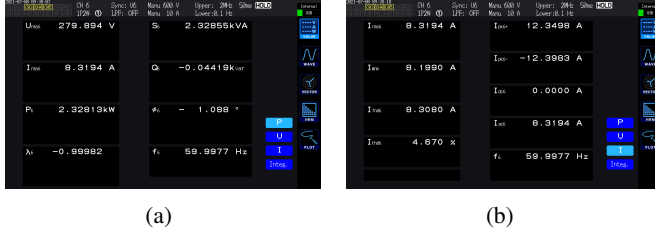
Fig. 8: (a) Power factor and (b) current THD at 100% load.
