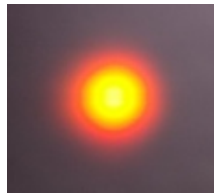
FIG. 7: Photograph of scatter from a white card for typical NOPA beam to display the near-TEM 00 spatial mode routinely achieved by the CPA-PFM-NOPA.
