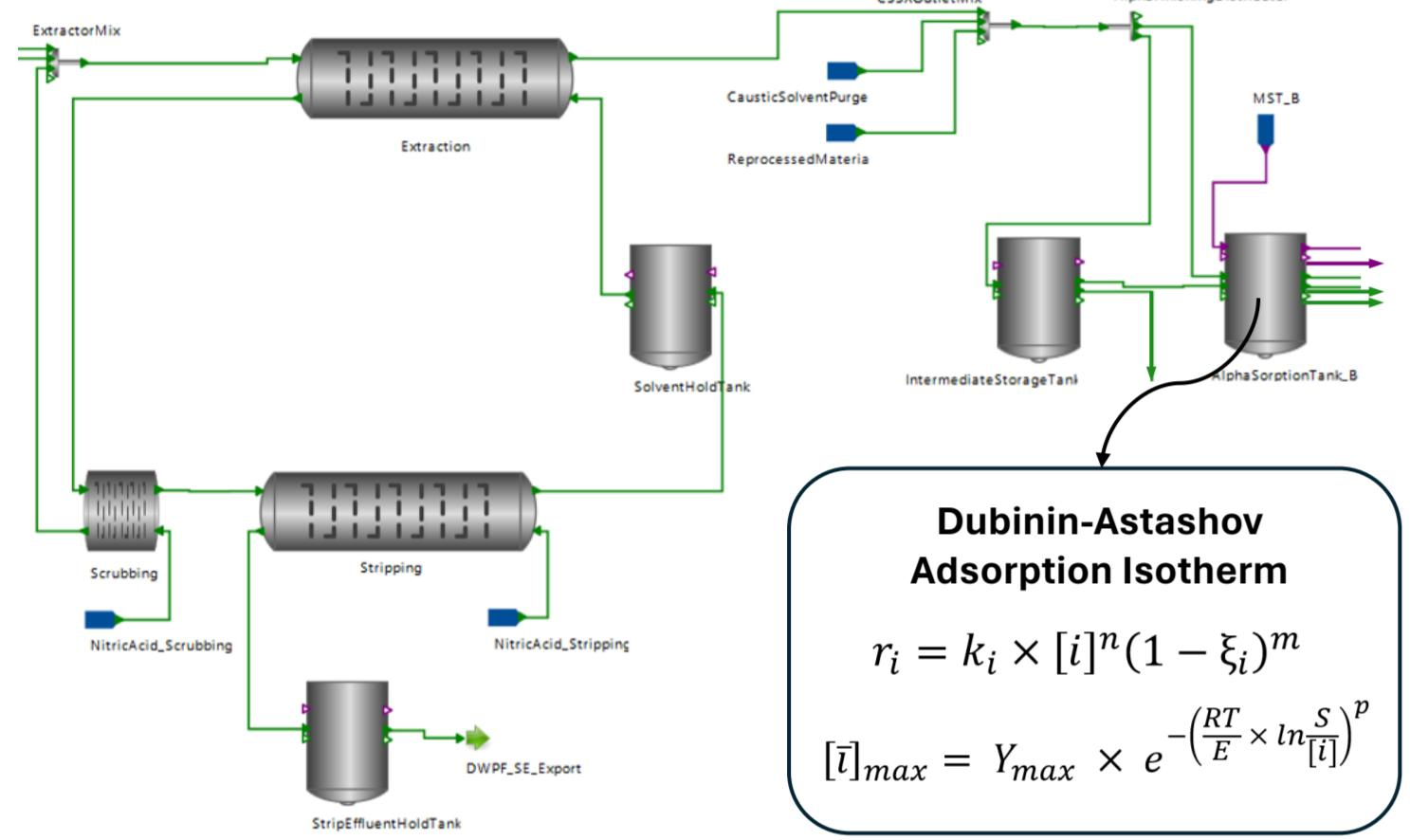
The TOM simulates material movement and chemical reactions at the Tank Farm (TF), Salt Waste Processing Facility (SWPF) and Defense Waste Processing Facility (DWPF).
