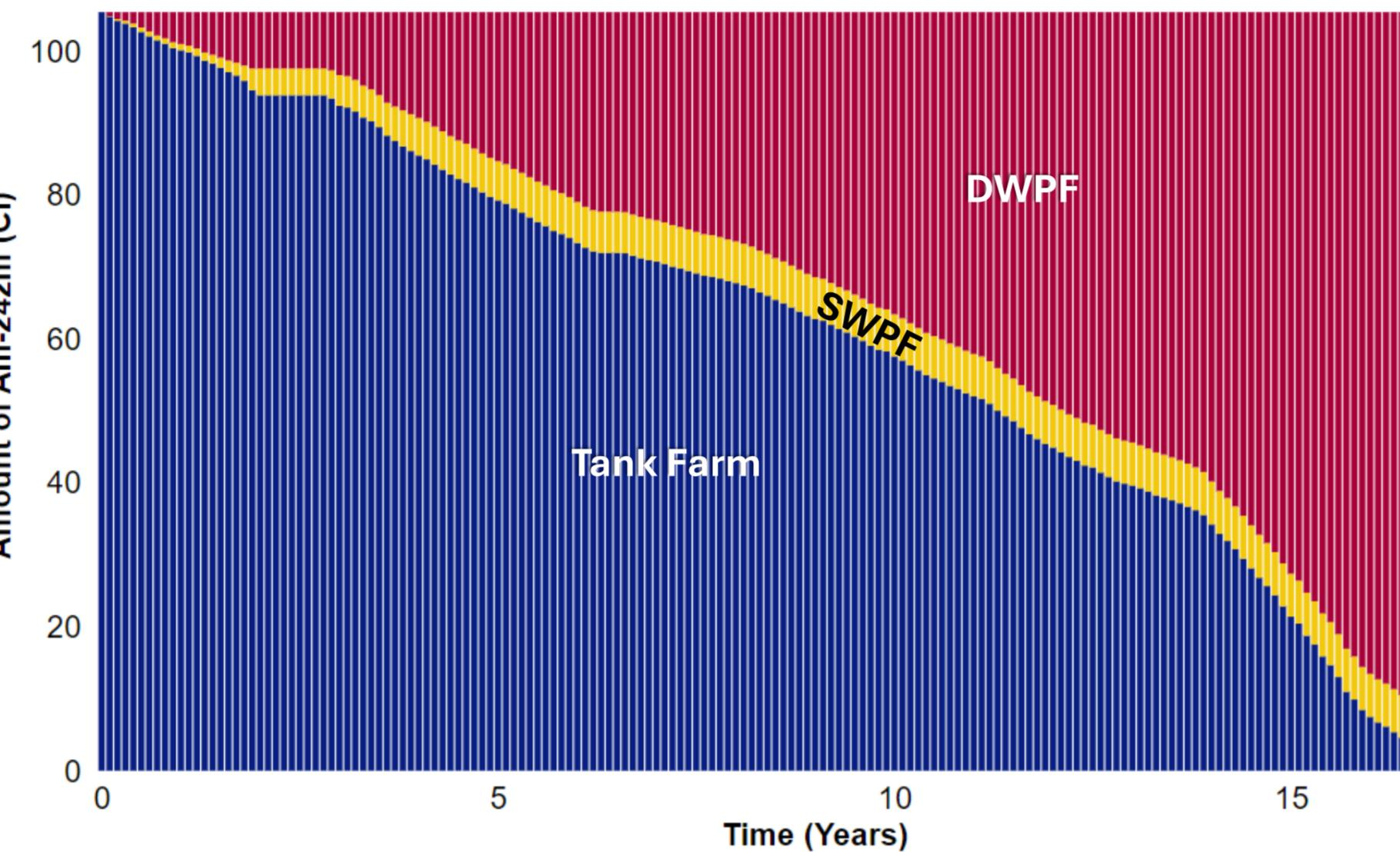
The figure above shows the movement of Am-242m between 3 key facilities across a 17-year simulation run. The above visual enables identification of material gain or loss in a simulation lifecycle.
