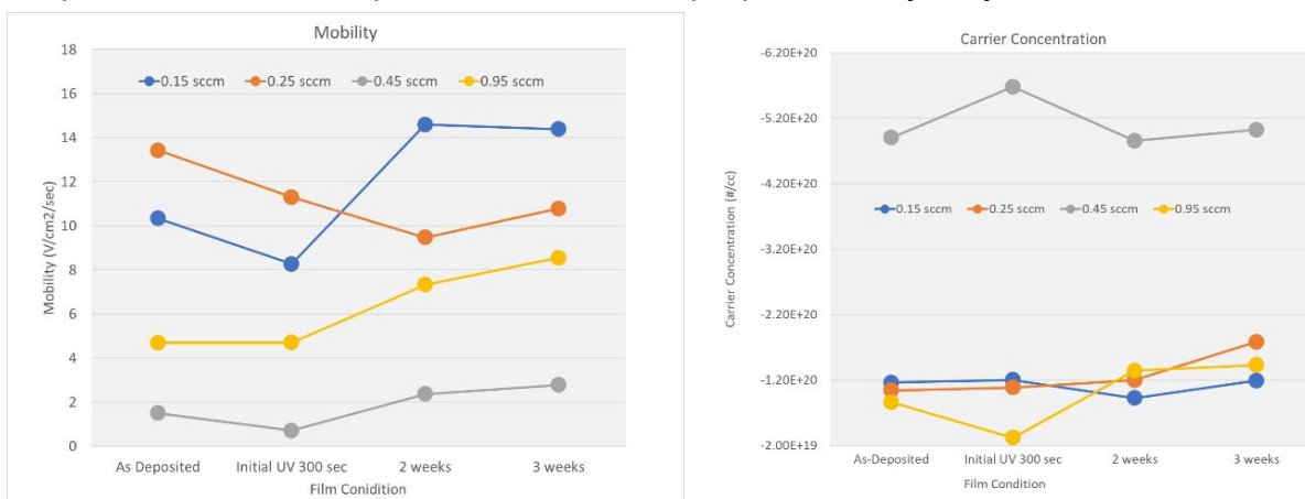
Fig. 30. ASU Gen 3 source ITO coatings on glass exposed to an accelerated aging test and then left in atmosphere for 3 weeks to determine ITO coating electrical stability.
