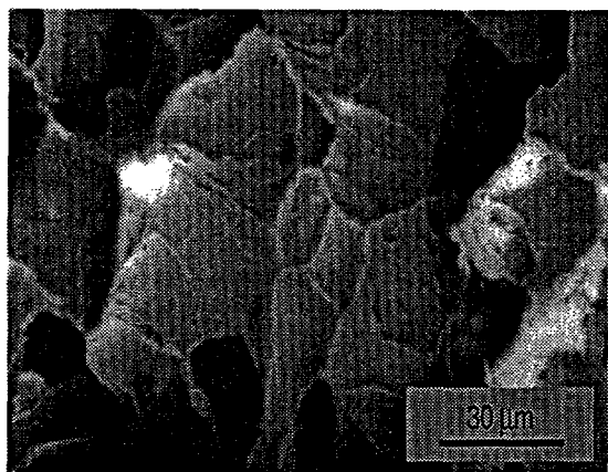
Figure 7. Fracture surface of tantalum spalled at 17 GPa peak pressure.
