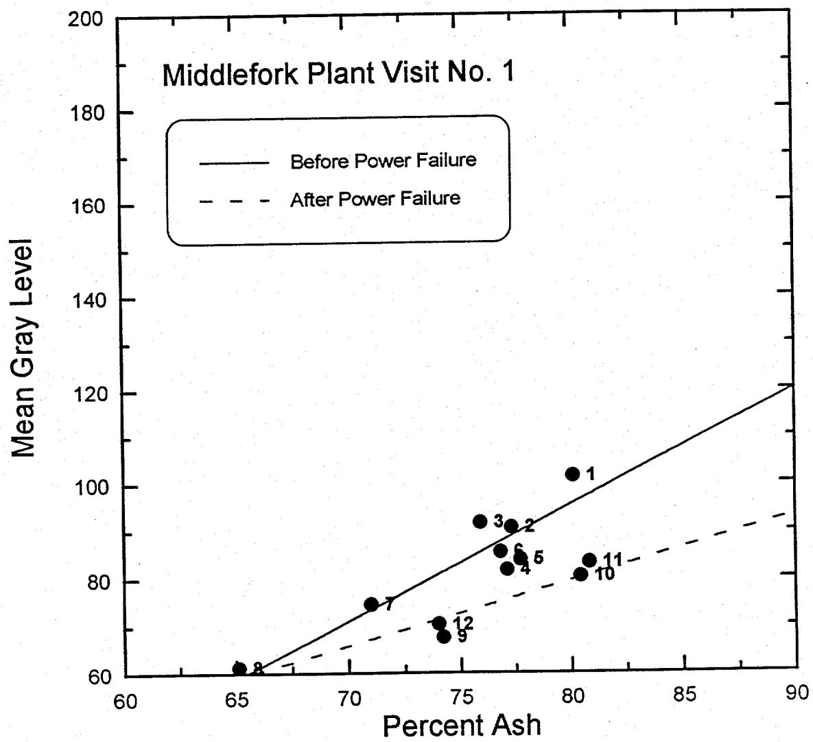
Figure 1. Mean gray level versus ash content for 12 samples collected during Middlefork preparation plant visit #1.
