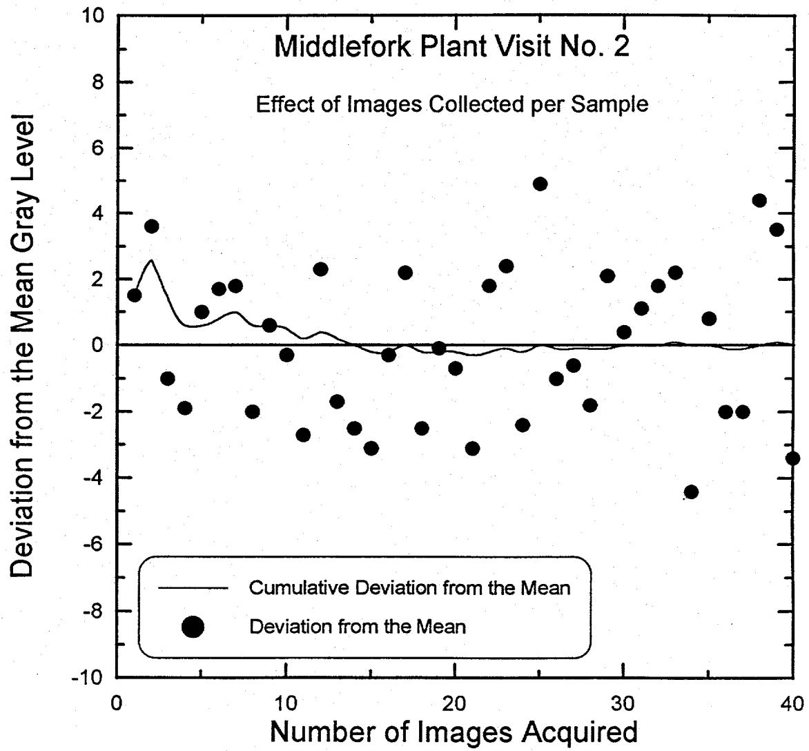
Figure 5. Effect of number of images collected per sample on the overall average mean gray level measured for a 76% ash slurry sample.
