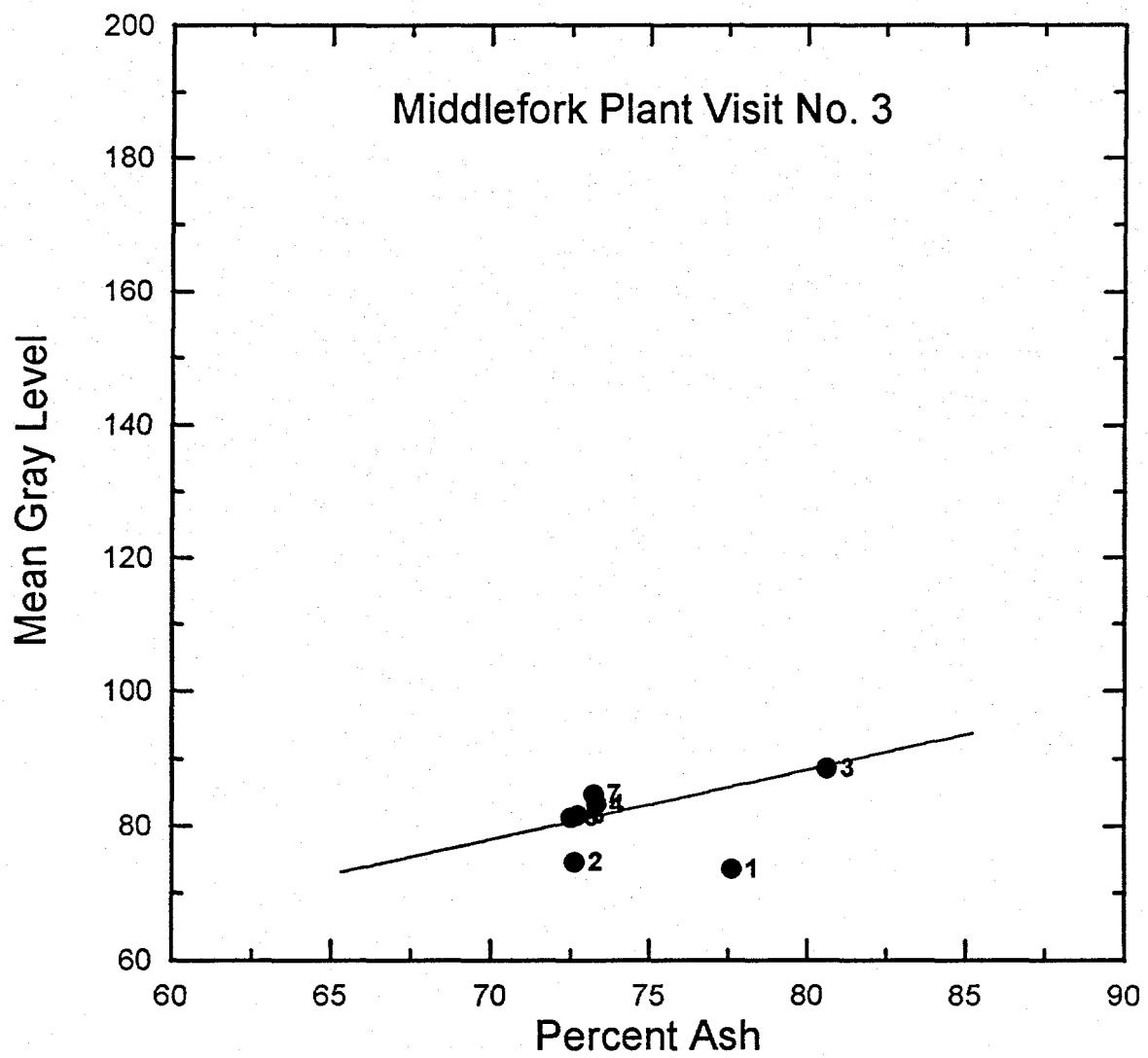
Figure 8. Mean gray level versus ash content for 7 samples collected during Middlefork preparation plant visit #3.
