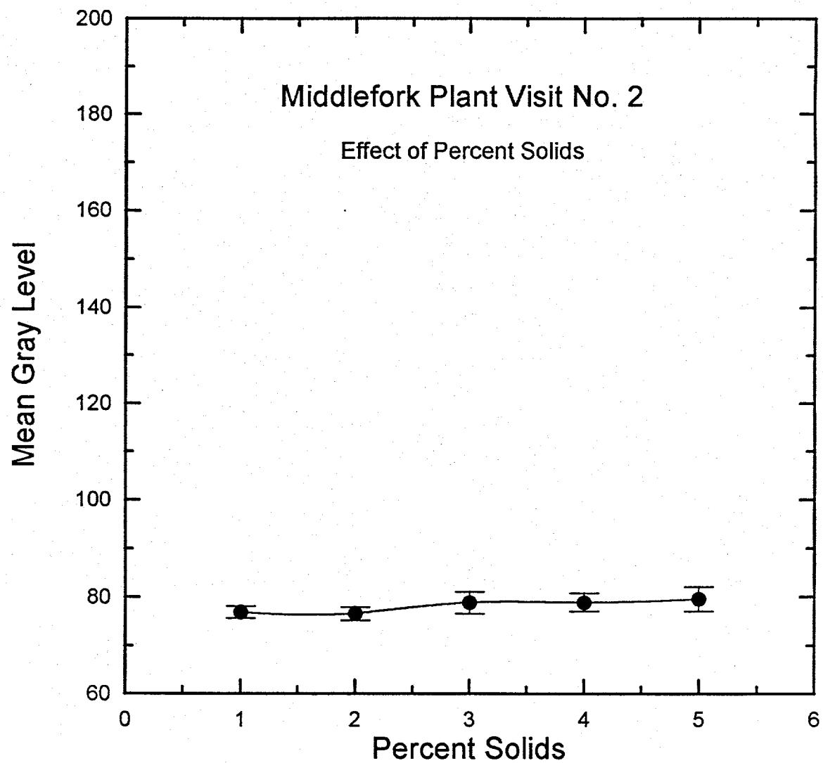
Figure 3. Effect of percent solids on mean gray level for a 76% ash slurry sample.
