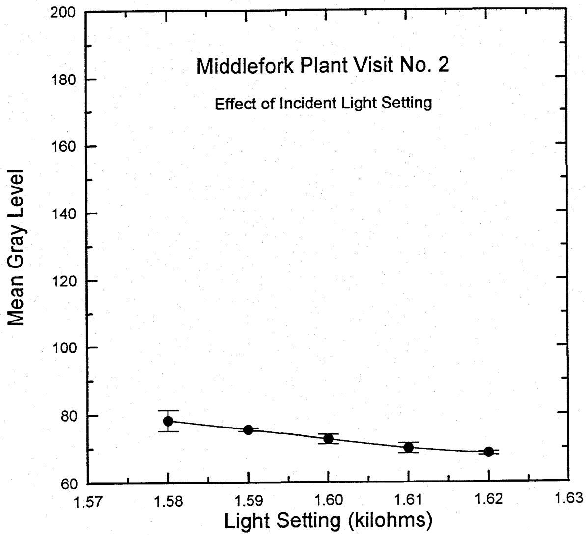
Figure 4. Effect of incident light intensity on mean gray level for a 76% ash slurry sample.
