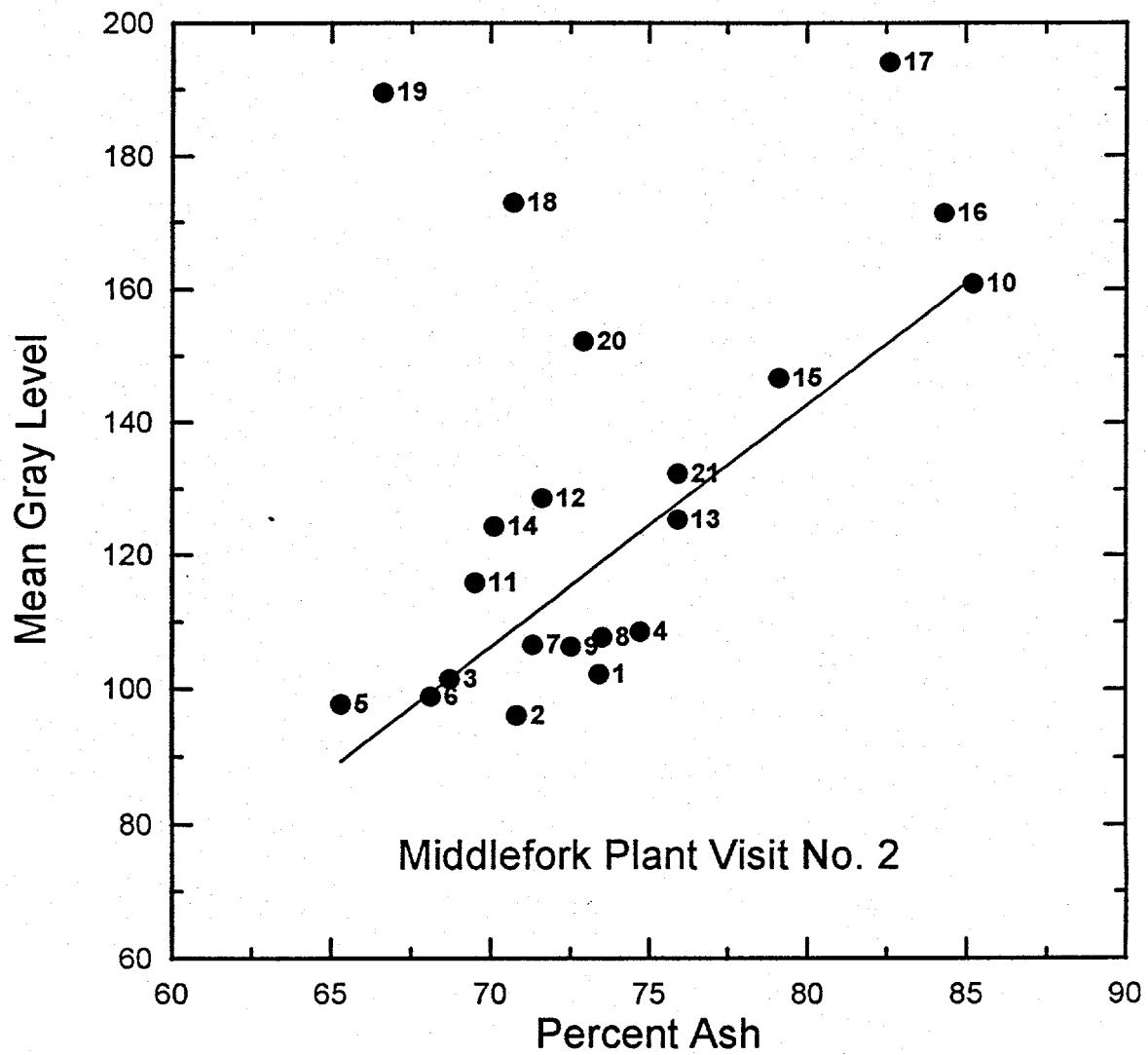
Figure 2. Mean gray level versus ash content for 21 samples collected during Middlefork preparation plant visit #2.
