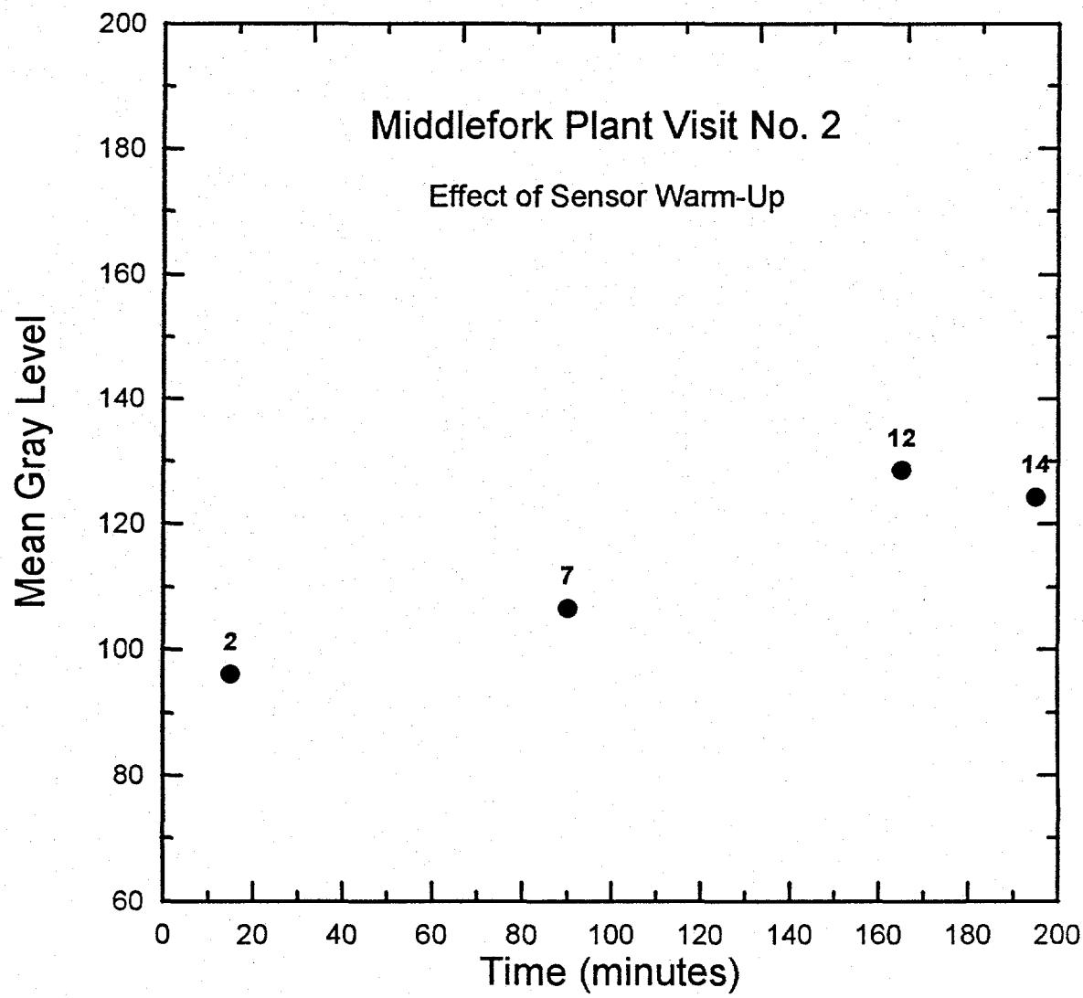
Figure 6. Mean gray level as a function of sample collection time for slurry samples with similar ash content and similar percent solids.
