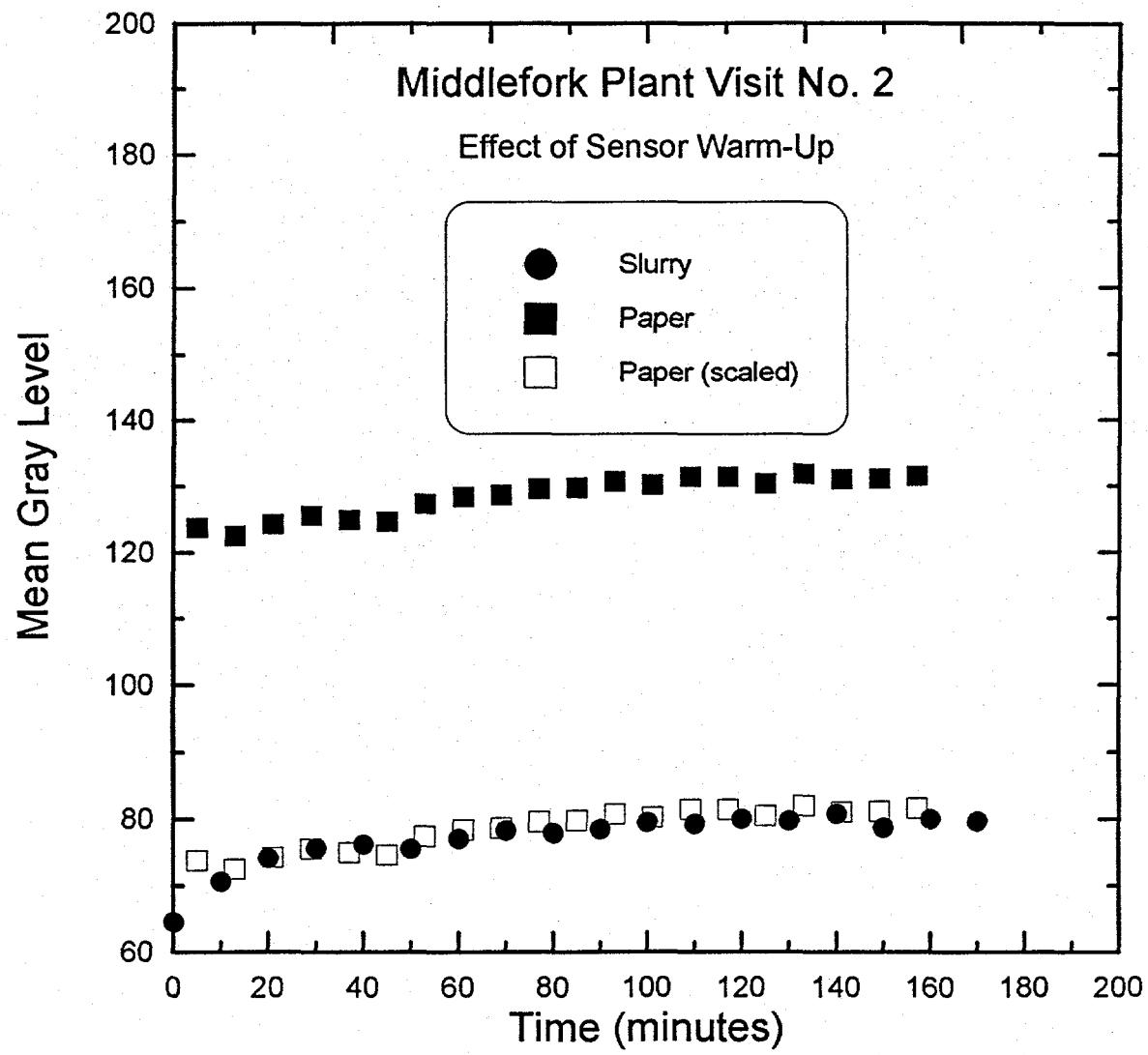
**Figure 7.** Effect of warm-up time on mean gray level values obtained using coal slurry and paper.
