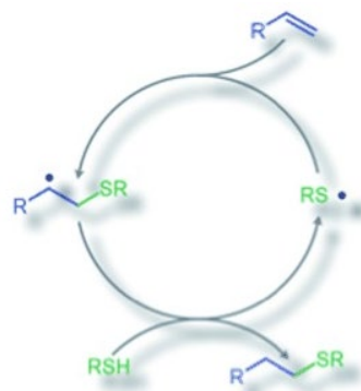
Scheme 1. Thiol-ene reaction scheme. Adapted from Hoyle et al 17 .
