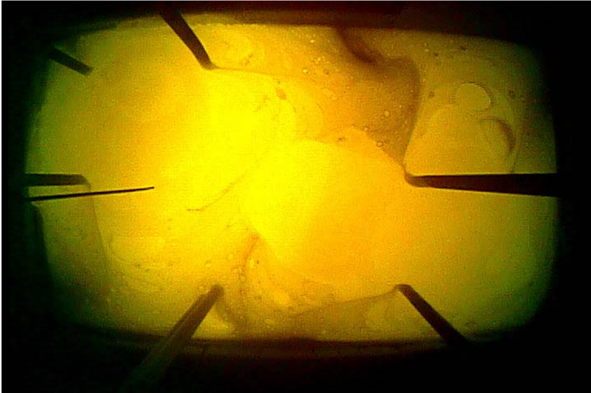
Figure 8. Still image of the 8" separation configuration at a high flow rate of 40 l/min for each nozzle at a depth of 20".
