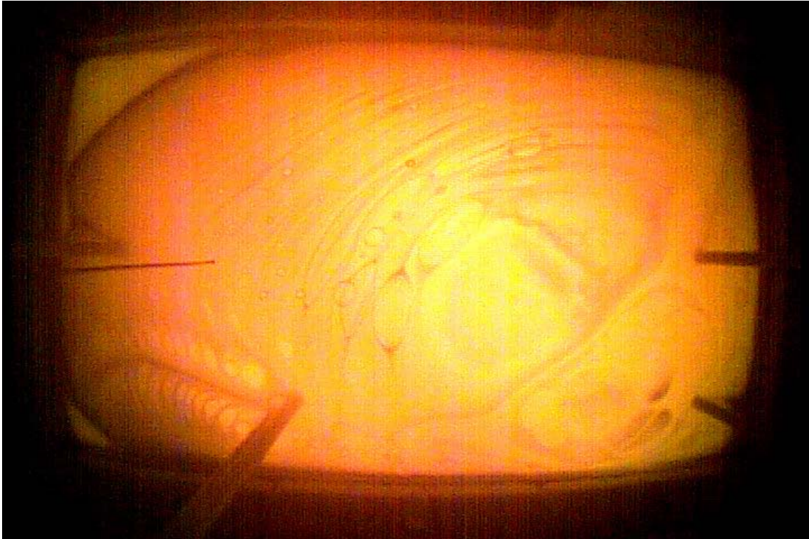
Figure 9. Still image of the bubbling for a double nozzle bubbler. The bubbler depth was 25" and the total flow was 32 l/min for the two nozzles.
