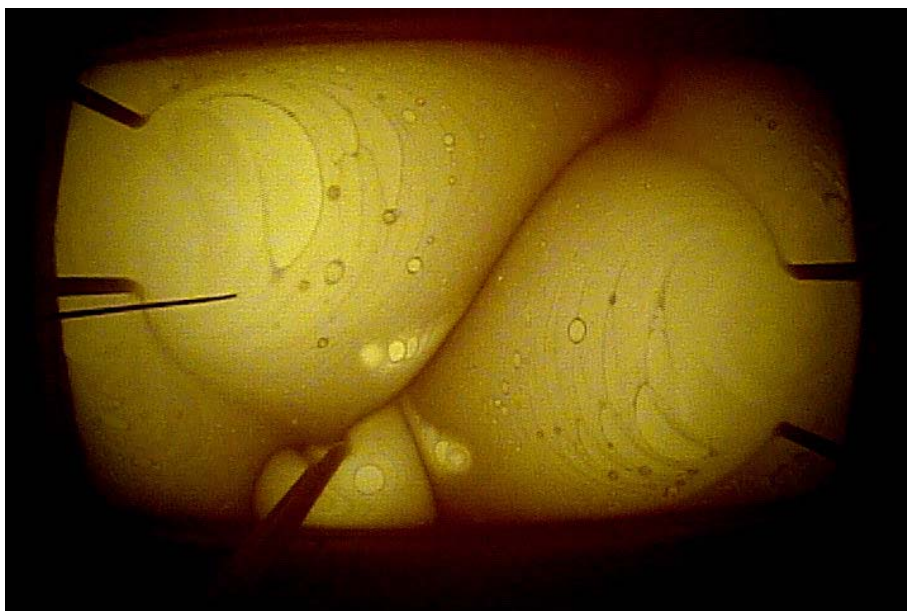
Figure 4. Still image from video of bubbling for two J bubblers in ports A3 and D1 with J's parallel to the electrodes and the nozzles 6" from the nearest wall.
