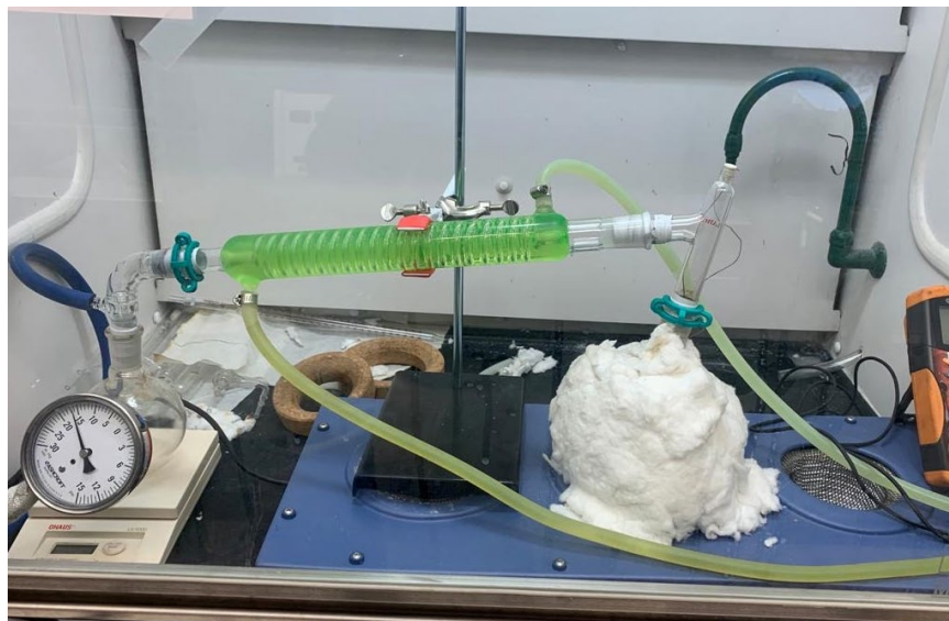
Figure 33: Upgraded vacuum distillation apparatus to accommodate low-temperature condensation of vapor distillate
