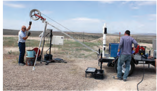
Setting a transducer in well PM-3 on August 8, 2022 (Central and Western Pahute Mesa Corrective Action Units 101/102)
