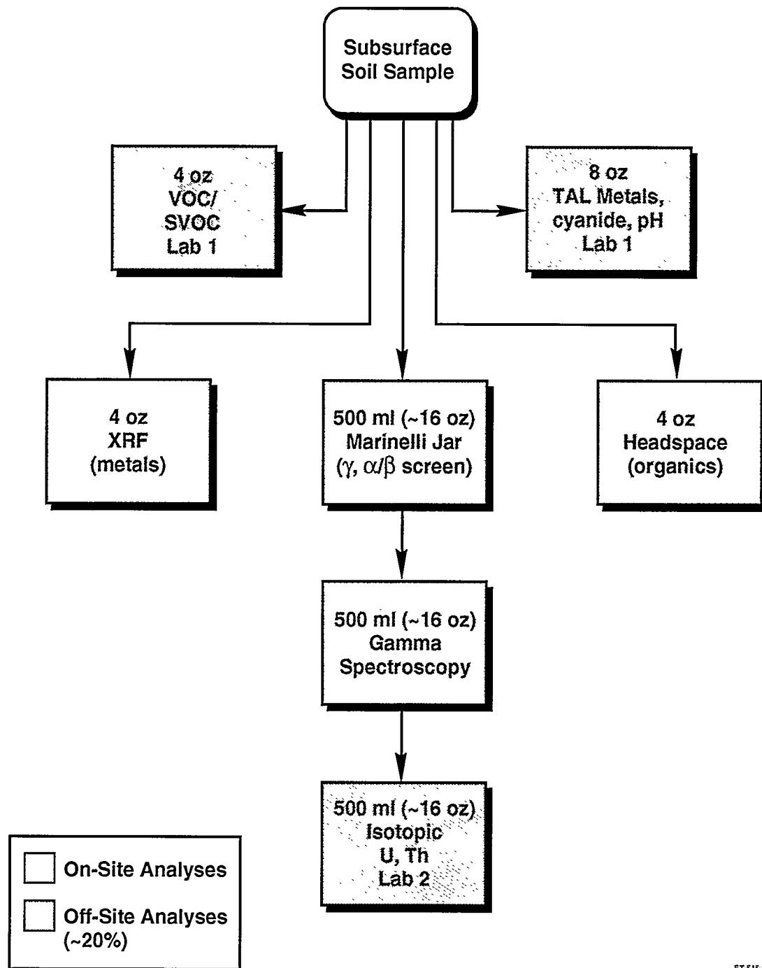
Figure 5. Flow diagram illustrating how splits from each subsurface soil sample were allocated for on-site field screening and off-site laboratory analyses.
