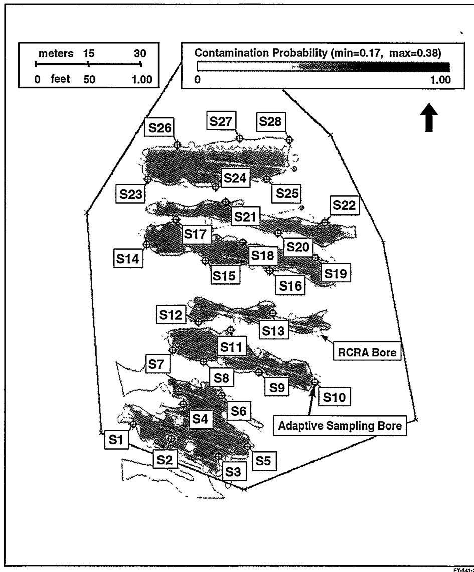
Figure 3. Plan view of RB-11 conceptual model with the locations for Adaptive Sampling and RCRA soil bores.
