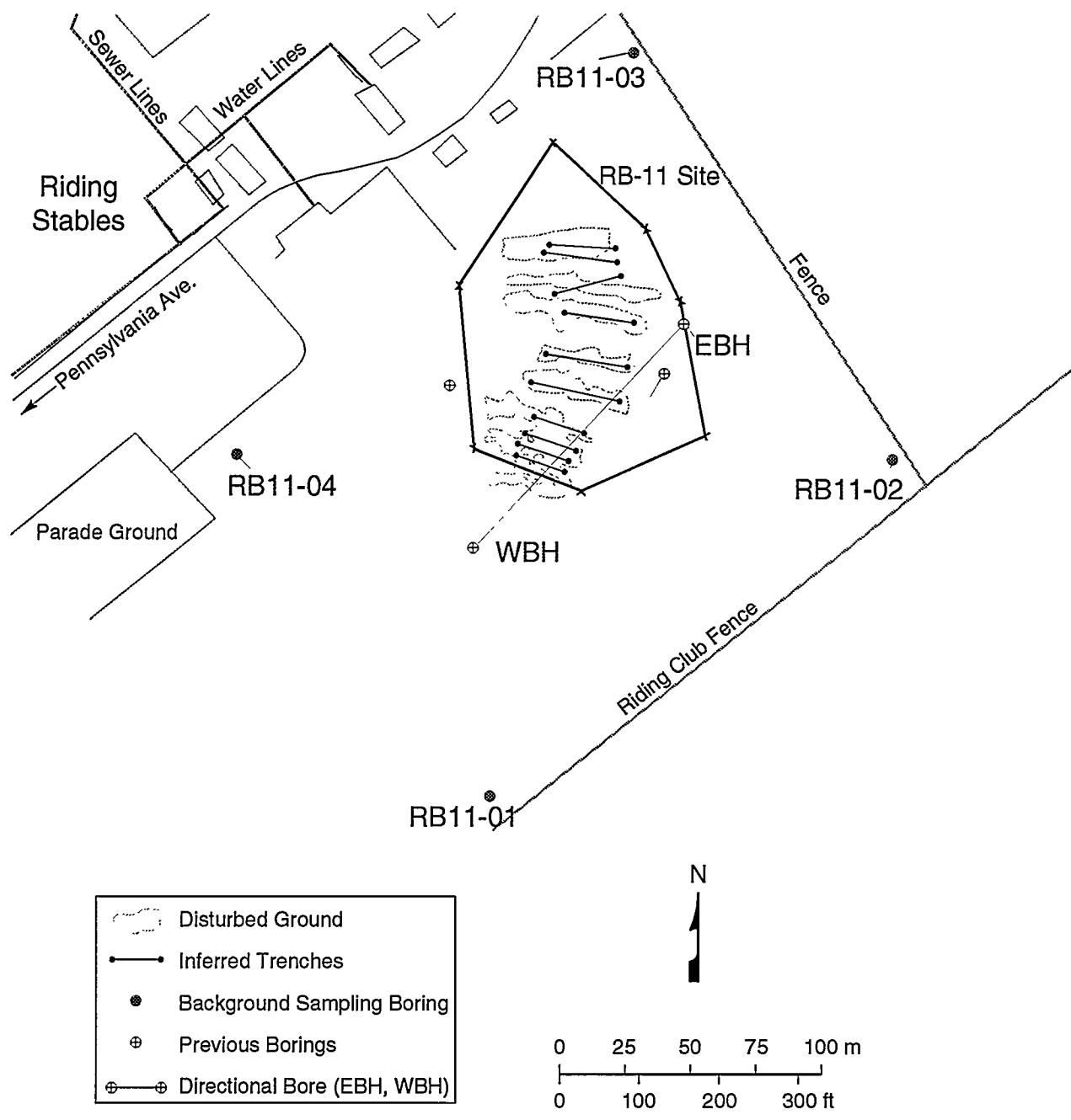
Figure 2. RB-11 Site showing infrastructure, inferred location of waste trenches and surrounding disturbed ground. Background sampling points are shown at perimeter (RB11-1 through RB11-4).
