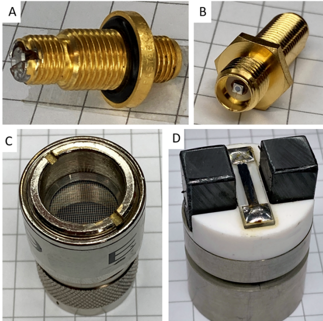
Figure 19. P&E detectors: A) diamond PCD, B) silicon diode C) XRD, and D) nickel bolometer.
