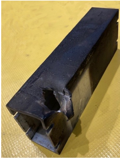
Figure 12. A “bullet” debris impact hole onto the calorimeter housing. The direction of the hole suggests that the impacting object was not part of the primary load hardware but likely came from another “ride-along” diagnostic test suspended above the load. The calorimeter data was corrupted by this impact.
