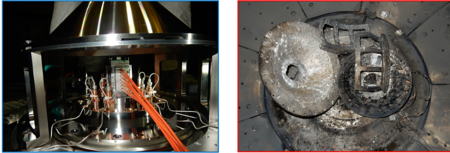
Figure 11. Left: A DMP load hardware set photo before the shot. Right: large pieces of the remainder of the hardware post shot (some physical rearrangement of the items prior to the photo occurred).
