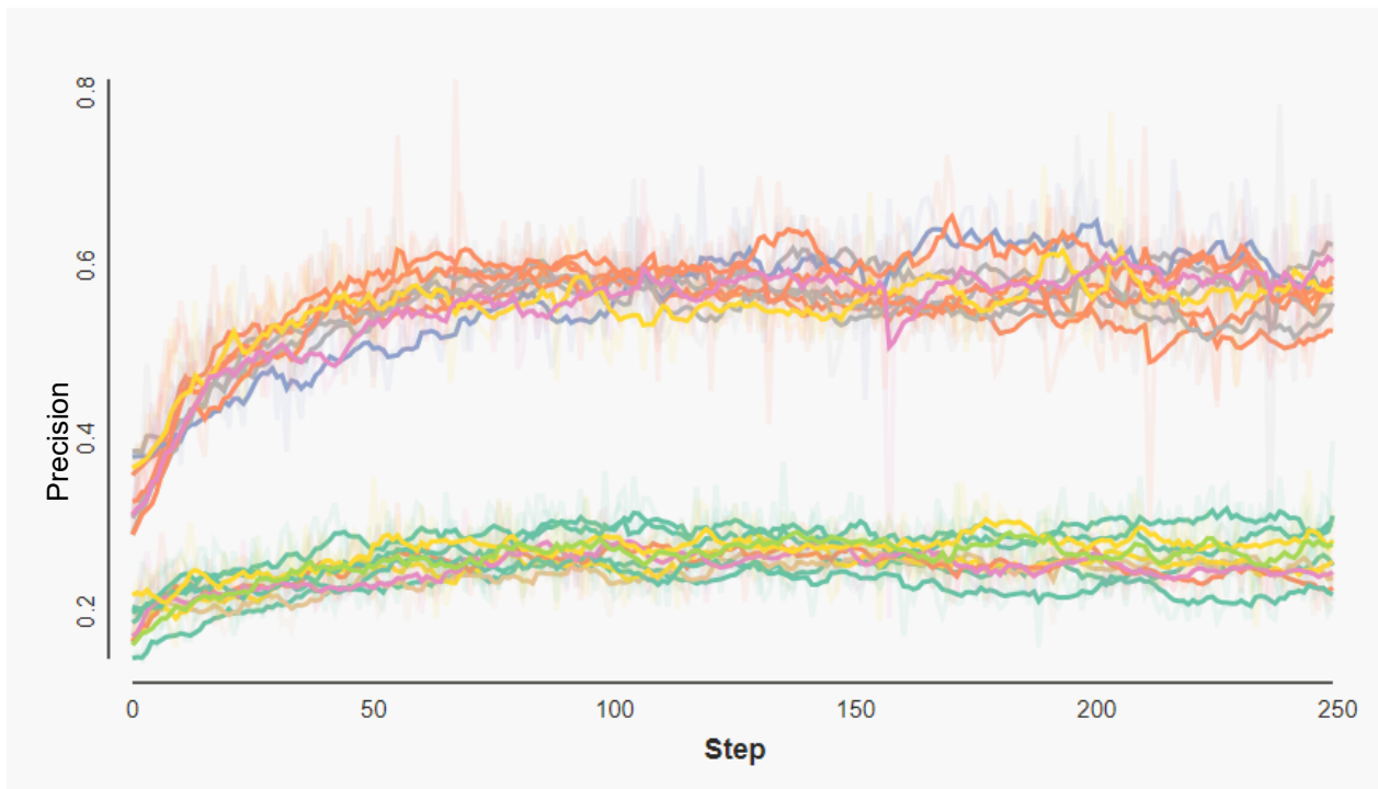
Figure 19. Precision scores from our image classification experiment show that image classification models trained with distractor objects (top cluster of red/orange lines) had higher precision than models trained without distractors using only background scenes as negative examples (bottom cluster of yellow/green lines).
