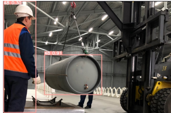
Figure 14. Example false positive detection results, in which the YOLO-v5s model identified a human and a 30B container as 48-type containers.
