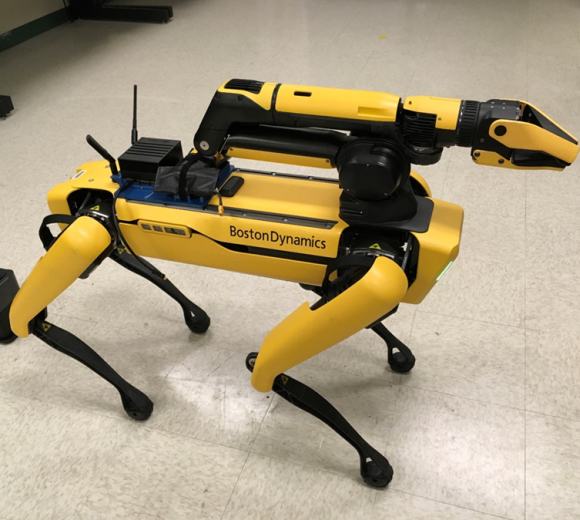
Figure 3: Spot with mounted Nvidia Jetson companion computer and GPU, complete with wireless connectivity.
