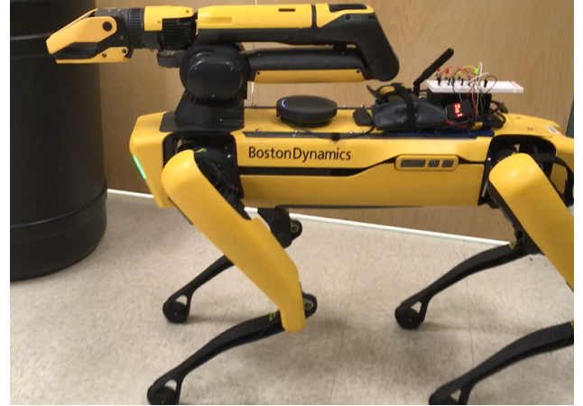
Figure 11: Spot with mic/speaker and prototype push button interface installed.
