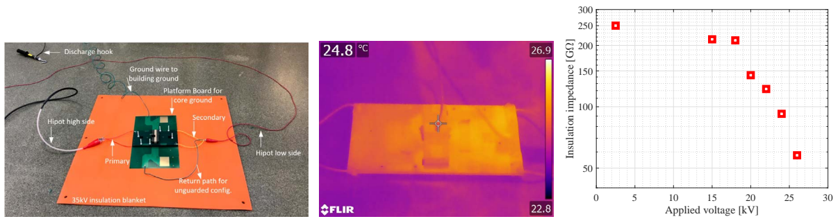
Figure 3: Hipot test setup and result data: (a) Photograph of the hipot testing setup with the device under test and connections from the PTS-75 hipot tester marked, (b) thermal image of the MV transformer with 26 kV applied between its primary and secondary terminals with grounded core segments, and (c) measurements of insulation impedances reported using the hipot tester across a wide range of applied voltages. Operating conditions : Ambient temperature : 21.9°C, Relative humidity : 10.10%, elevation from sea level : 5,675 ft.
