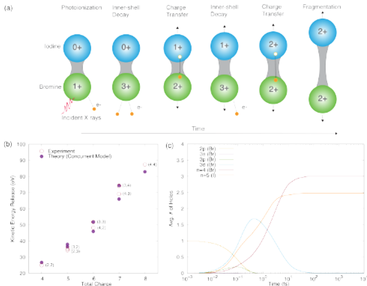
FIG. 6. (Color online) (a) Concurrent model of inner-shell deexcitation and fragmentation dynamics of IBr. (b) Kinetic energy distributions of various ion fragmentation pairs of IBr measured at 13486 eV in coincidence with Br K\alpha emission. The open and filled circles are the experimental data and calculated results from a concurrent model, respectively. (c) Average number of vacancies in each subshell of Br and the valence shell of I as a function of time, starting from a vacancy in 2p of Br.
