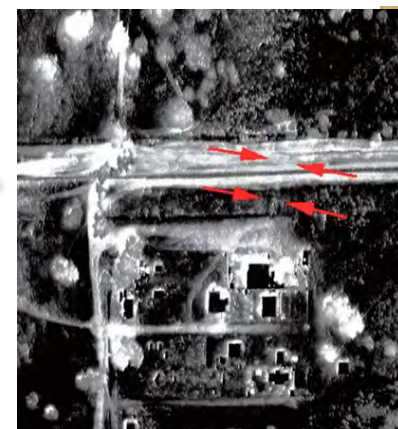
Heat flow model predicted optimum acquisition times to maximize thermal contrast of subsurface void
