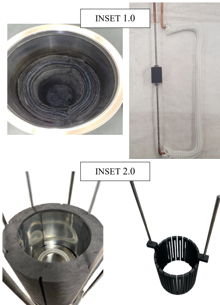
Figure 1. Insulation and heating element of INSET 1.0 (top) versus INSET 2.0 (bottom) [4].
