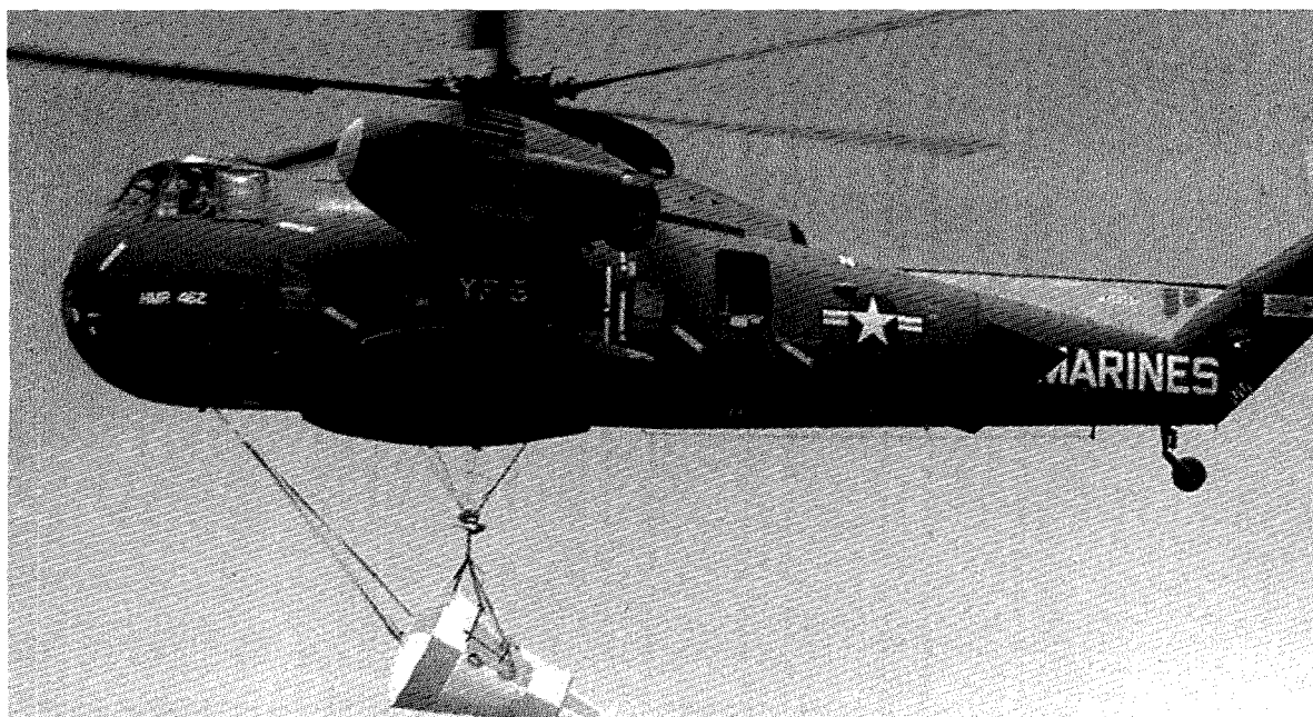
A helicopter raises a NASA Mercury space capsule for test drops in Salton Sea. Sandia's crew provided photographic coverage of the drops and capsule-recovery assistance.
