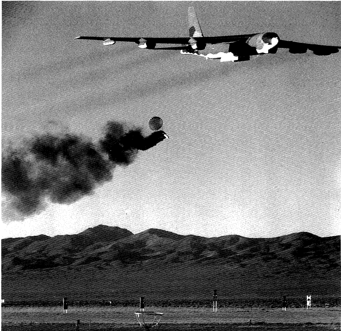
A 1977 test drop of a laydown B77 bomb by a B52 aircraft onto the range's concrete target.
