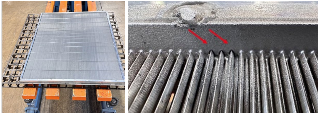
Figure 63: (Left) Full aluminum HX prototype before brazing at Diesel Radiator; (Right) Post-braze inspection revealed small gaps near tube trailing edges.
