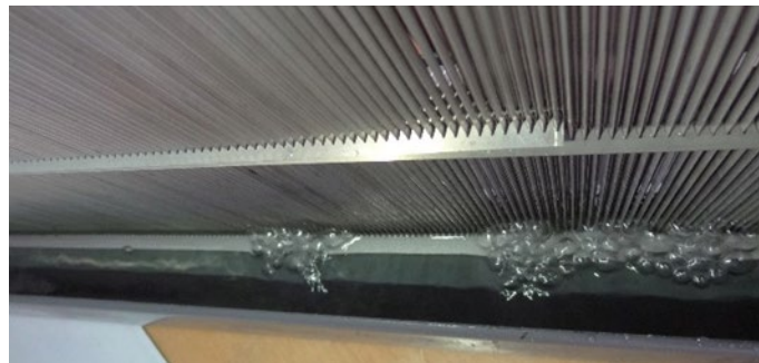
Figure 64: Full aluminum HX prototype with multiple post-braze leaks.
