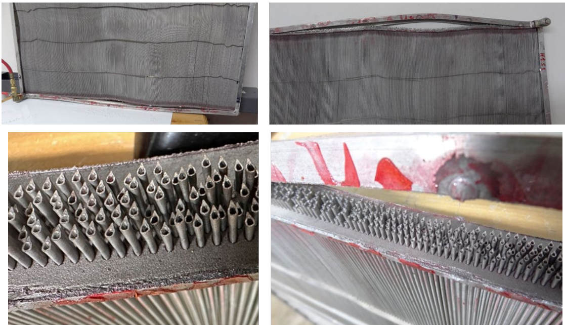
Figure 68: Aluminum HX post-pressure test: (Top) Tank-header joint failure; (Bottom) Poor brazed interfaces between tube-header and header-tank.
