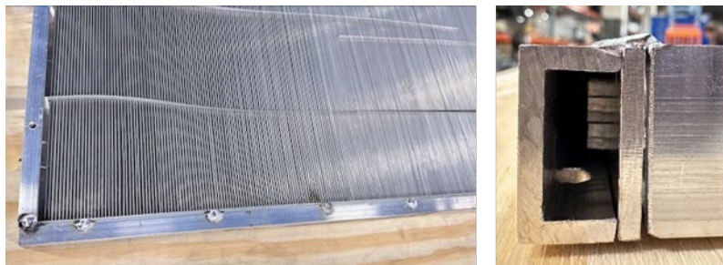
Figure 62: Aluminum HX pre-braze: (Left) Complete frame; (Right) Open tank ends.
