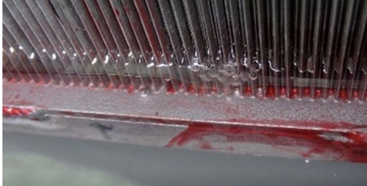
Figure 67: Adhesive leak repair and pressure test #2 showing small leaks.
