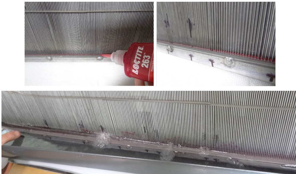
Figure 66: Adhesive leak repair #1: (Top) Adhesive application; (Bottom) Leak test.
