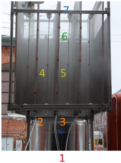
Figure 67: Locations of thermocouples in lab cooling tower collector (left) and corresponding average plume temperatures overlaid on curve of predicted liquid water content (right).
