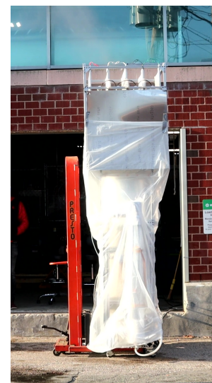
Figure 19: Lab cooling tower test with plastic shroud preventing mixing of ambient air with plume until the plume leaves the collector.
