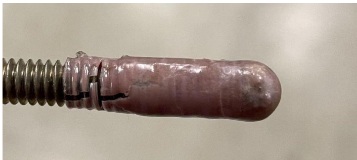
Fig. 5 Salt sample after 9 hours of U chlorination in Test #2.
