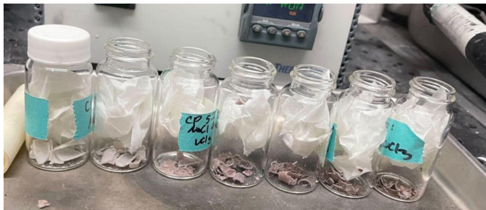
Fig. 2 The salt samples taken during Test #1 displayed chronologically according to chlorination time from left to right
