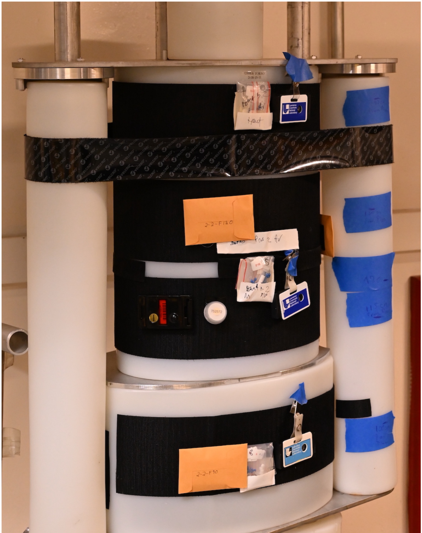
Figure 2.1: BOMAB phantoms were mounted on custom aluminum exposure stands. The blue tape markers on the right indicate different heights above the floor. From top to bottom, the markers are at 145, 130, 120, 115, and 100 cm above the exposure room floor.
