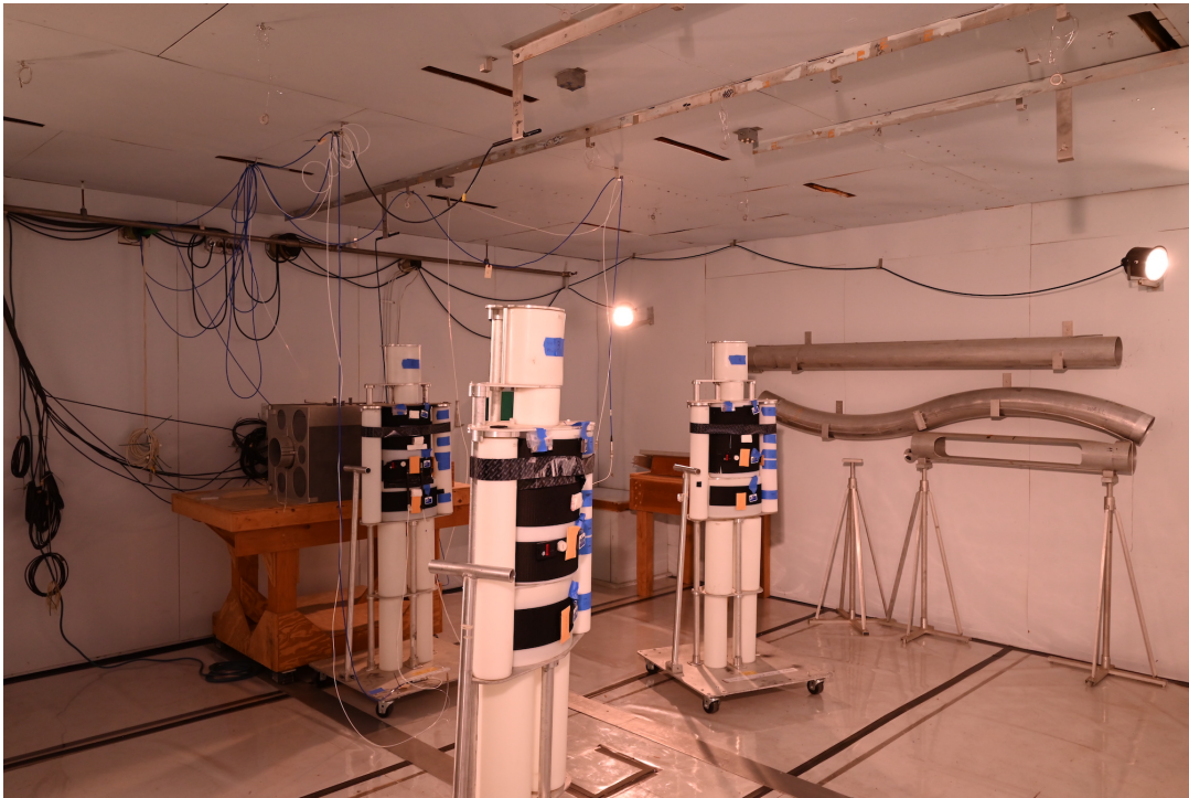
Figure A.3: BOMABs placed at position 3, 4, and 8 in ER1.
