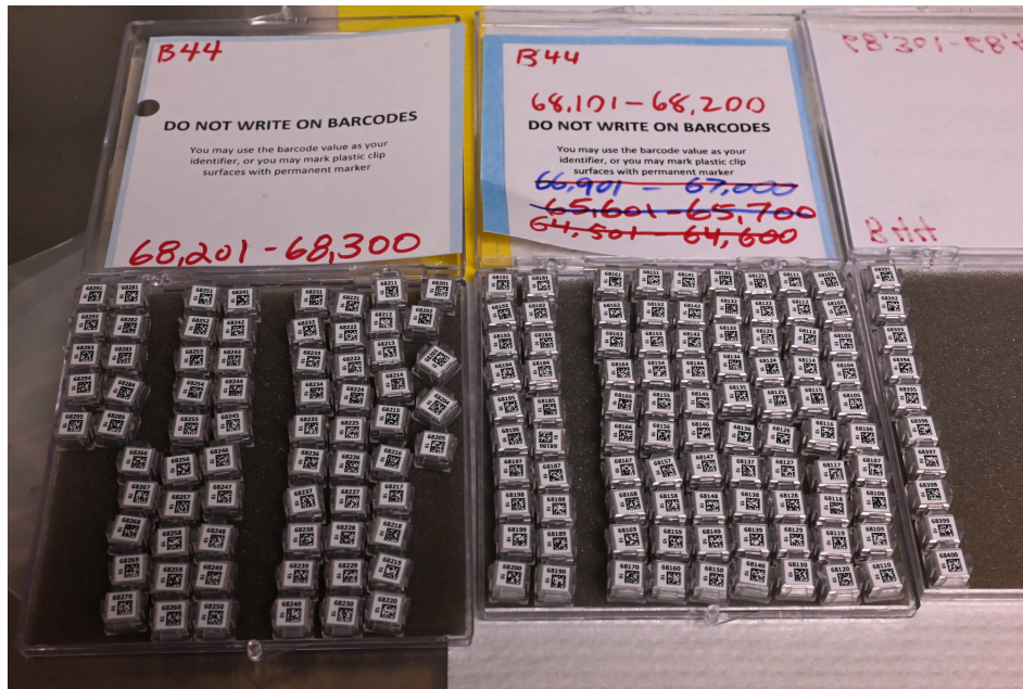
Figure 2.5: An assortment of \text{CaF}_2 TLDS used for the photon dose measurements at different distances.
