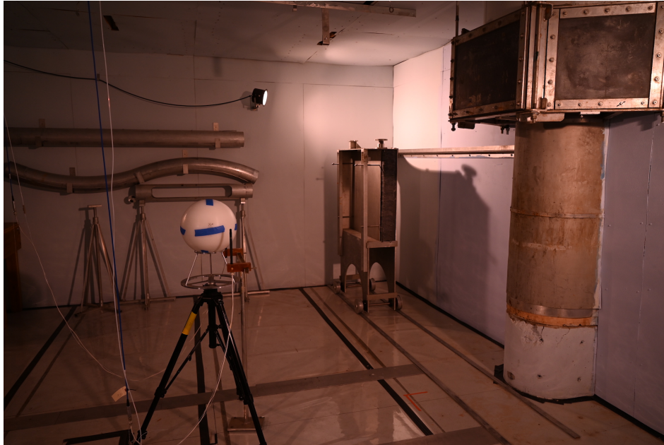
Figure 2.4: LLNL PNS sphere sitting on an aluminum stand and mounted on top of a tri-pod in ER1. The semi-circle portion of the wall is a cadmium liner (filter). The room walls are painted with a gadolinium paint. The purpose of the liner and paint is to reduce the number of thermal neutrons in the AFFRI leakage spectrum.
