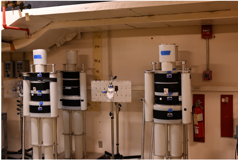
Figure 2.2: Three BOMAB phantoms and a free-in-air aluminum stand with dosimeters mounted on them. The dosimeters on the BOMAB phantoms were mounted at 100, 120, and 145 cm above the exposure room floor. The dosimeters on the free-in-air aluminum plate stand were mounted between 115 and 130 cm above the exposure room floor.
