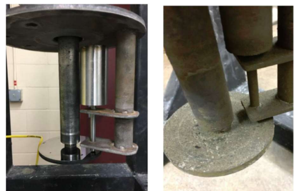
Figure 2: H230 disk, NiWC3b pin before and after test (left); H230 disk, NiWC3b pin after test (right)
