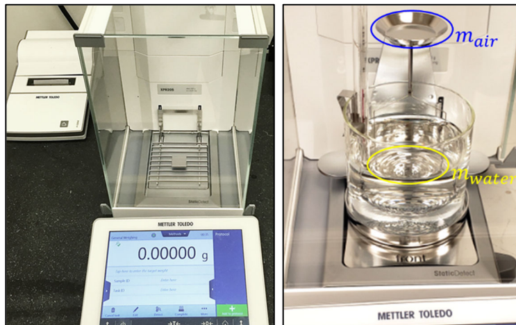
Figure 11. Analytical balance and density measurement kit.
