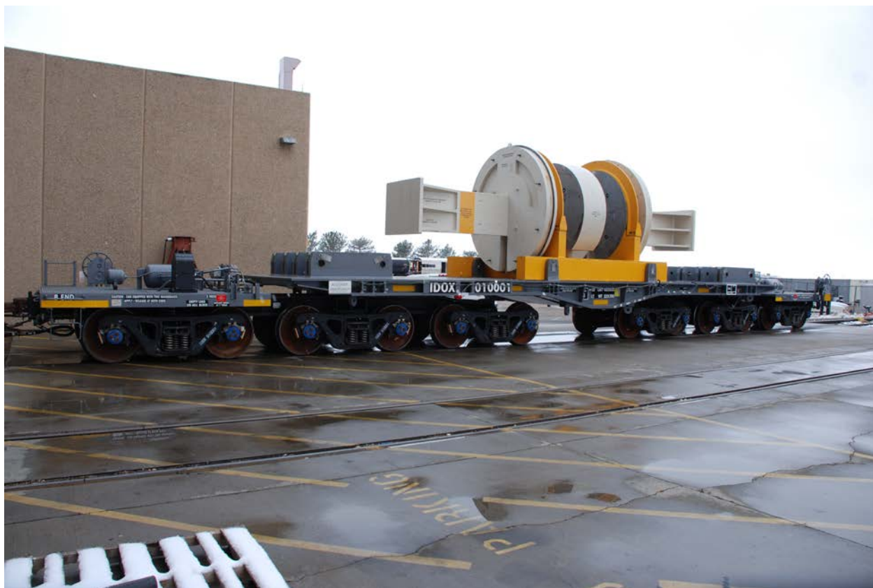
Figure 11. Atlas Railcar with Test Weights
