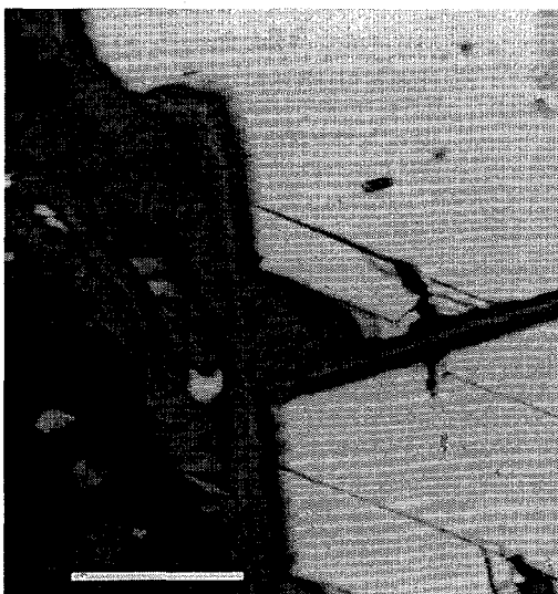
Fig. 4: Backscattered-electron image of sphalerite grain with feathery tertiary phase along surface and in fracture. Scale bar: 25 \mu m.
