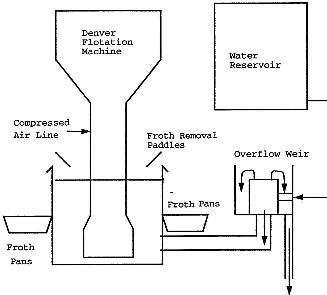
Figure 1. Schematic diagram of the conventional flotation cell showing the motorized froth scrapers and the pulp level control. Froth paddle speed = 19.5 rpm. Cell volume = 2.75 liters. Impeller speed = 1150 rpm.
